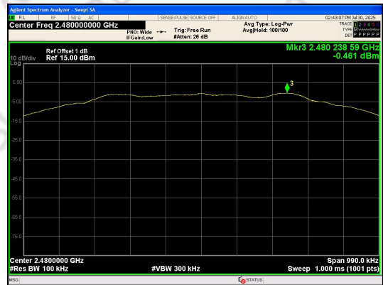
In-Band Reference Level BLE 1M_Channel 39
