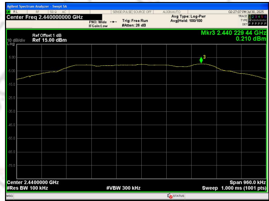
In-Band Reference Level BLE 1M_Channel 19
