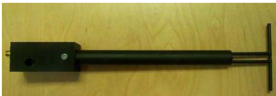
Figure 1 – MVG COMOSAR Validation Dipole
