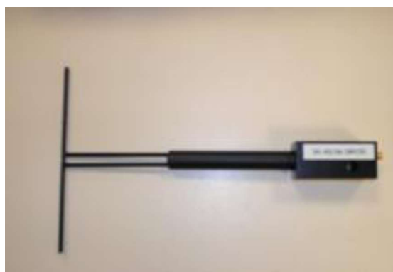
Figure 1 – MVG COMOSAR Validation Dipole
