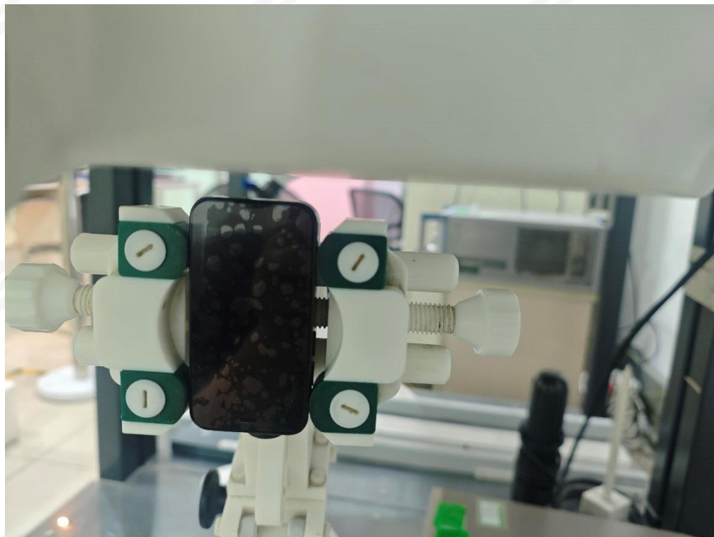
Body Top side(separation distance is 10mm)
