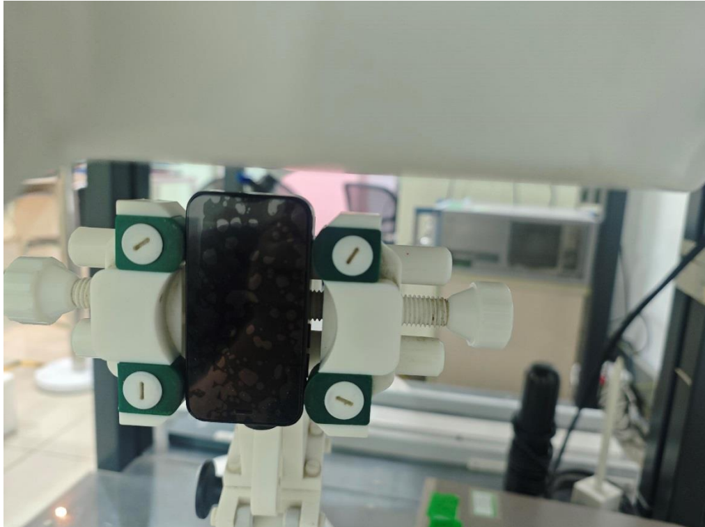
Body Top side(separation distance is 10mm)
