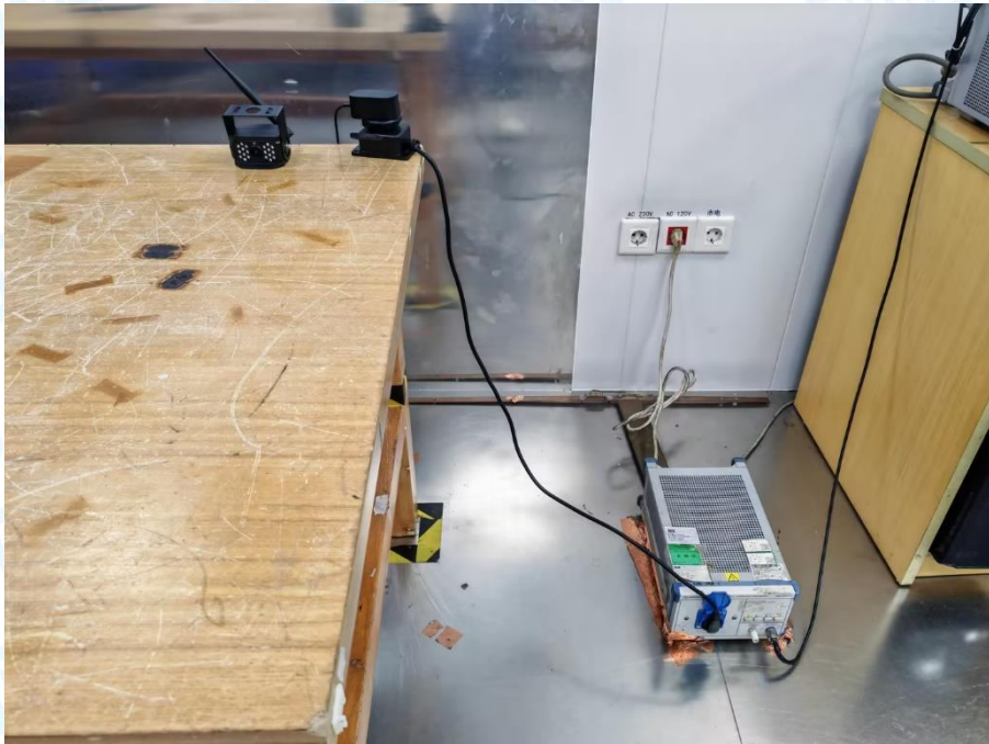
Photo of Setup for Radiated Emission (30MHz~1GHz)
