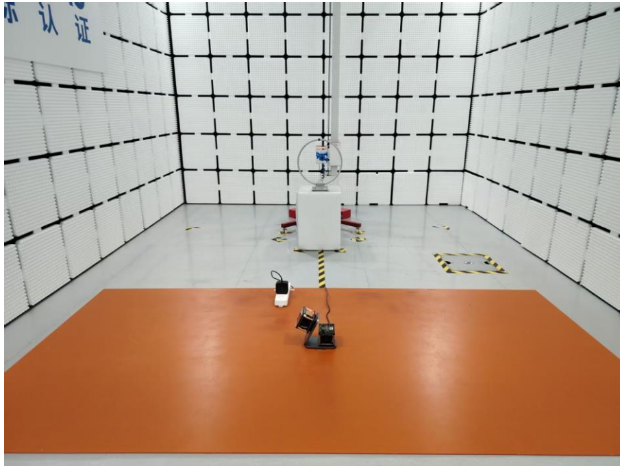
Radiated Emission Above 30MHz
