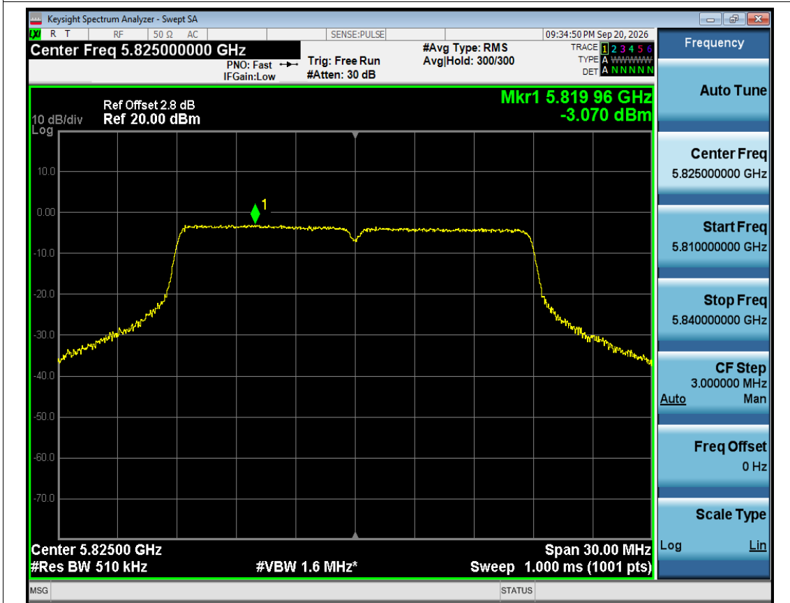
PSD NVNT n20 5825MHz Ant1
