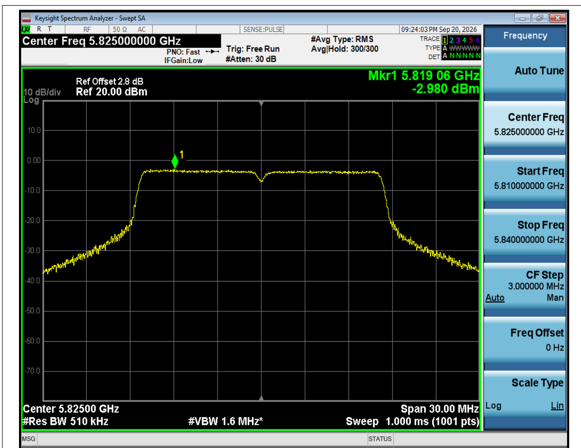
PSD NVNT a 5825MHz Ant1
