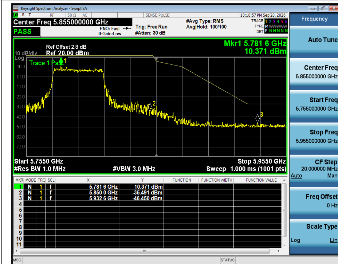
Band Edge NVNT ax40 5795MHz High Ant1
