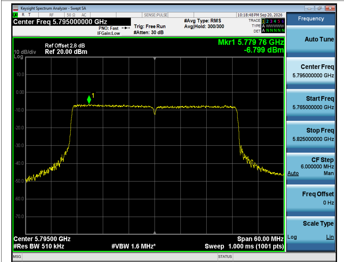
PSD NVNT ax40 5795MHz Ant1
