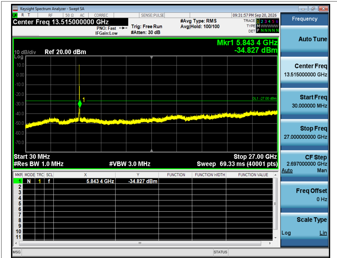
Tx. Spurious NVNT n20 5785MHz Ant1 Emission
