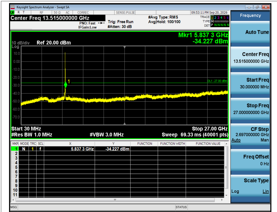
Tx. Spurious NVNT ax20 5785MHz Ant1 Emission
