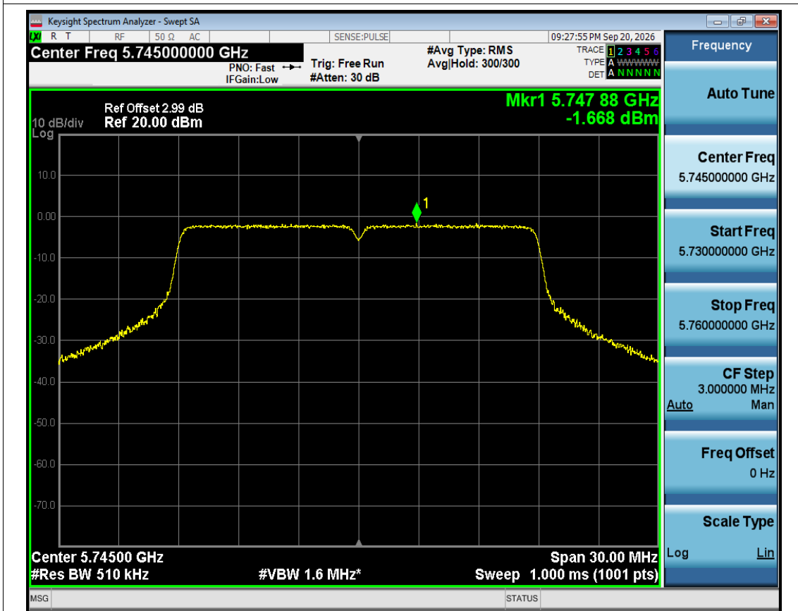
PSD NVNT n20 5745MHz Ant1
