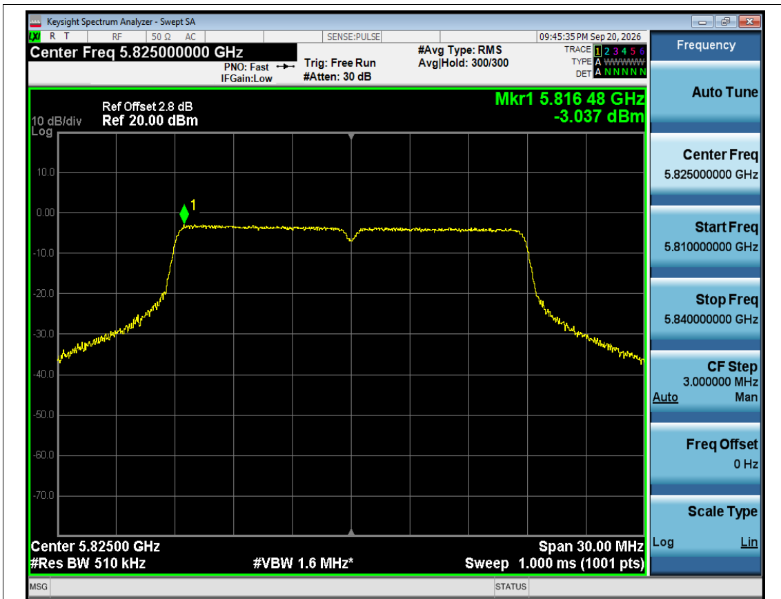
PSD NVNT ac20 5825MHz Ant1
