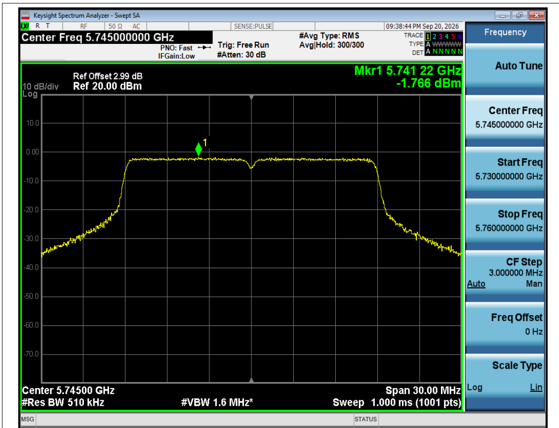
PSD NVNT ac20 5745MHz Ant1
