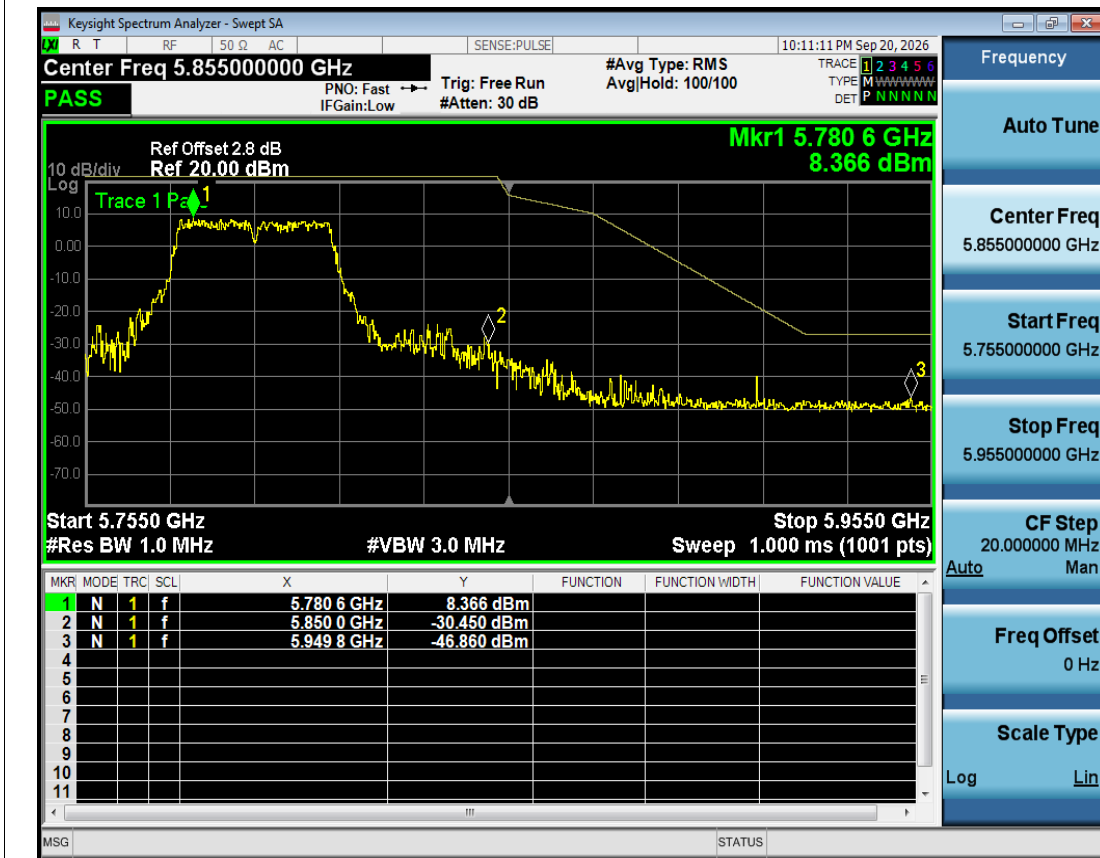
Band Edge NVNT ac40 5795MHz High Ant1
