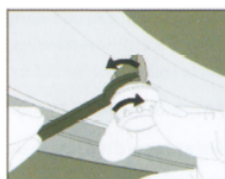
d. Tighten the sensor and tighten the anti-theft nut counterclockwise with a wrench
