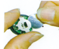
Remove the original battery and install a new battery
