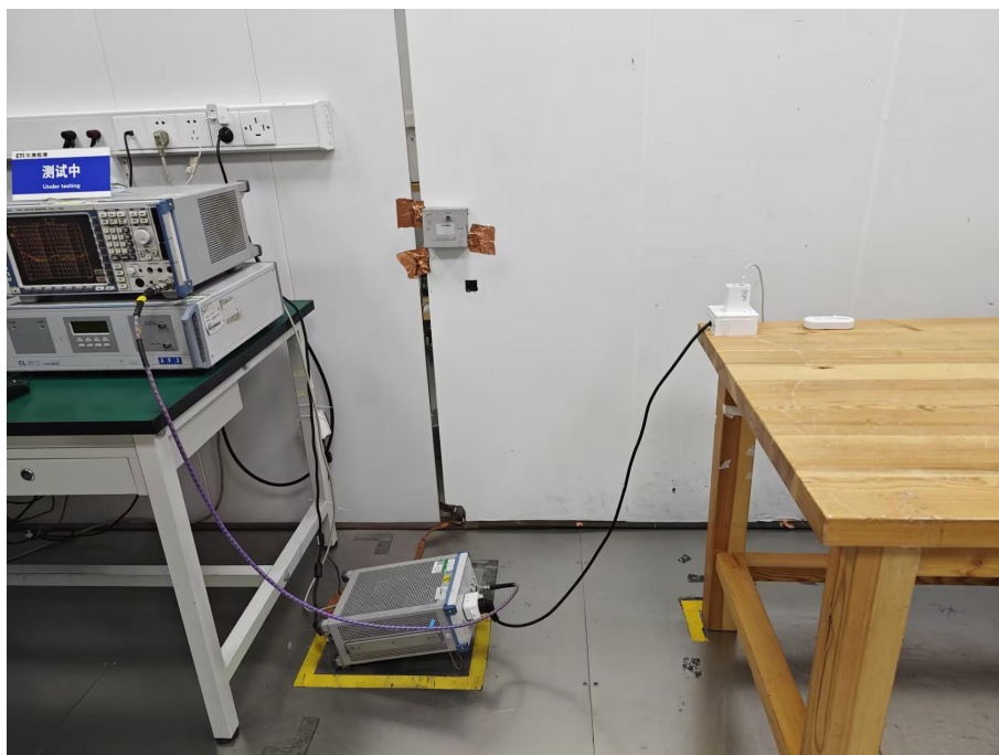
Conducted Emissions Test Setup
