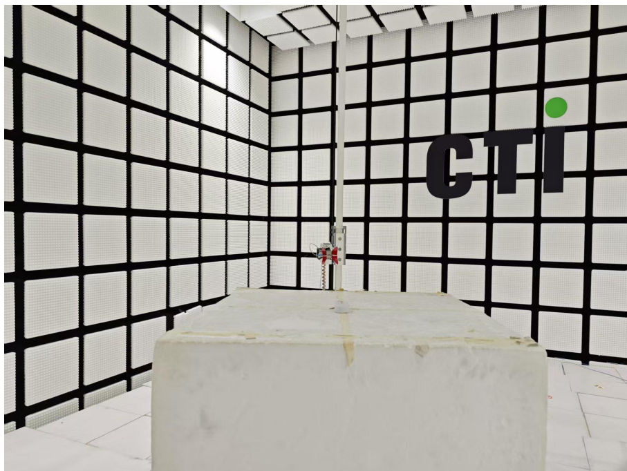
Radiated spurious emission Test Setup-2(Above 1GHz)
