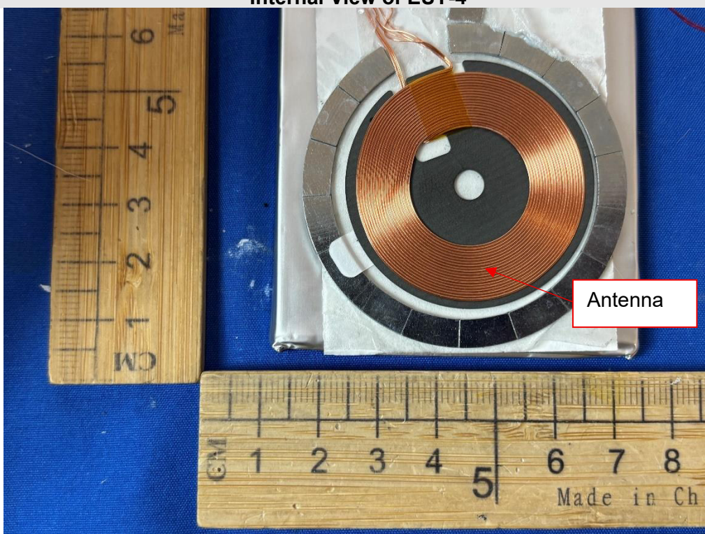
Internal View of EUT-4
