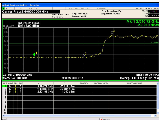
Out Of Band Emission(Left) 8DPSK_3-DH5_Channel Hopping
