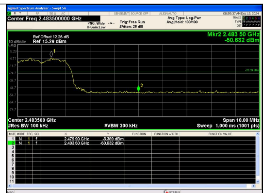
Out Of Band Emission(Right) 8DPSK_3-DH5_Channel Hopping
