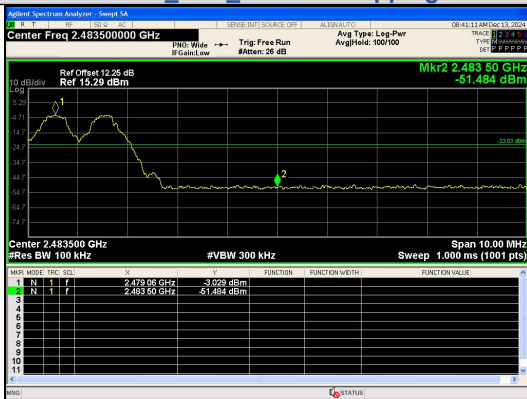
Out Of Band Emission(Right) GFSK_DH5_Channel Hopping
