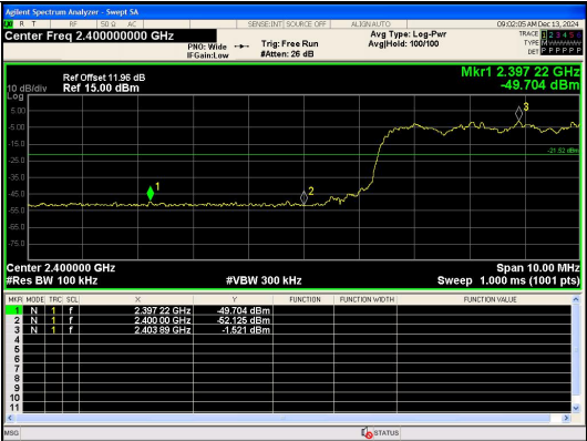
Out Of Band Emission(Left) 8DPSK_3-DH5_Channel Hopping
