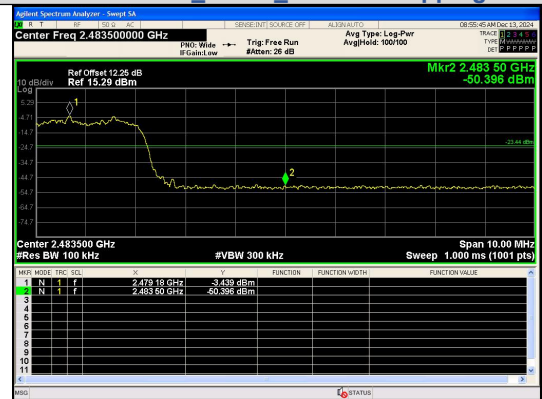
Out Of Band Emission(Right) \pi/4 DQPSK_2-DH5_Channel Hopping
