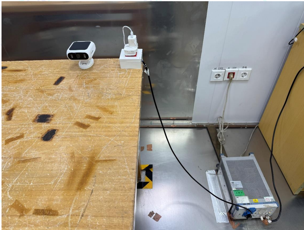
Radiated Emission Test Setup-Below 1G
