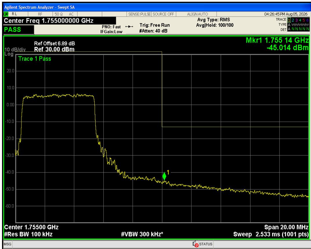
Band4 QAM16 BW=15MHz Channel=20025 RB Size=27 Position=#0
