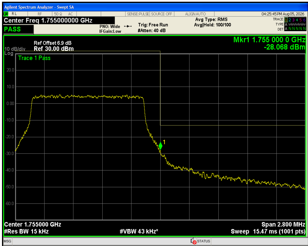
Band4 QPSK BW=3MHz Channel=19965 RB Size=15 Position=#0
