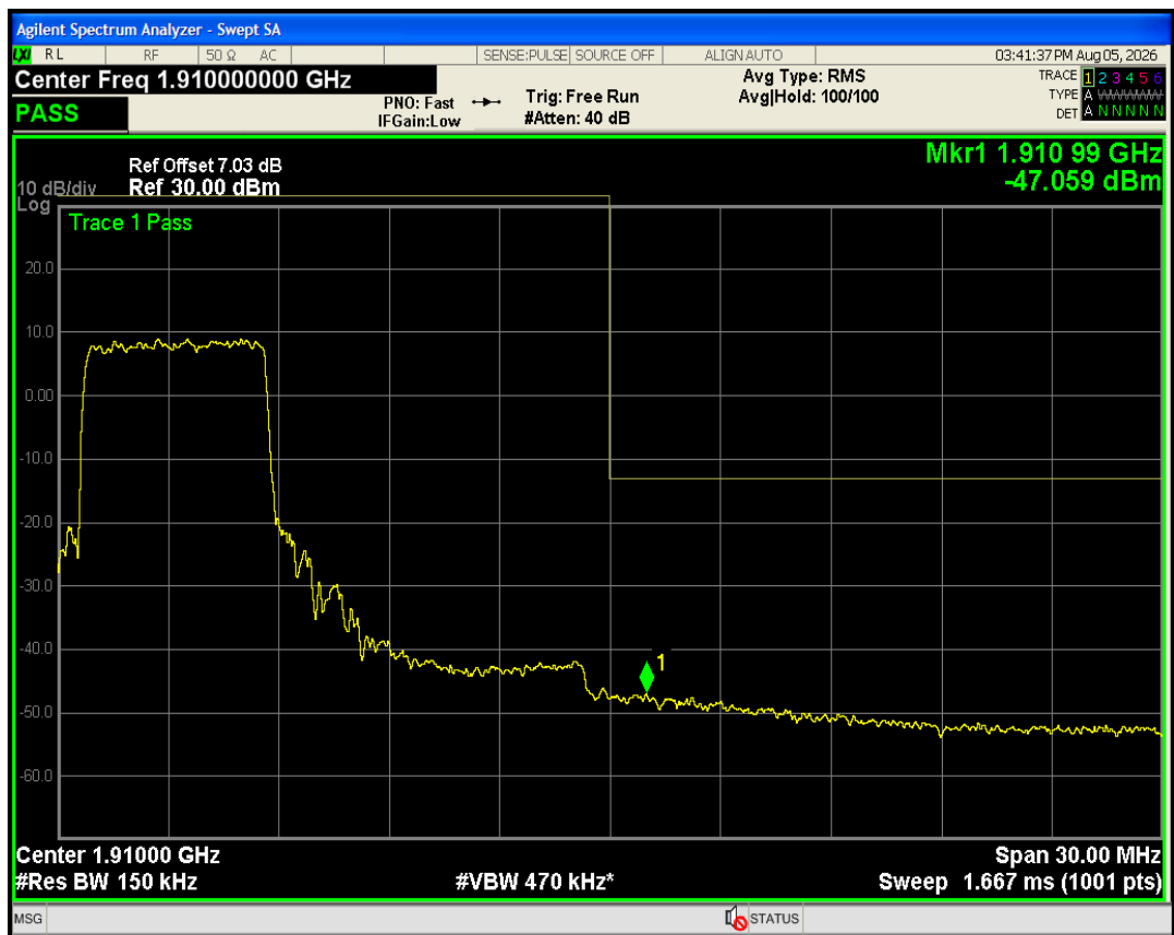
Band2 QPSK BW=15MHz Channel=19125 RB Size=75 Position=#0
