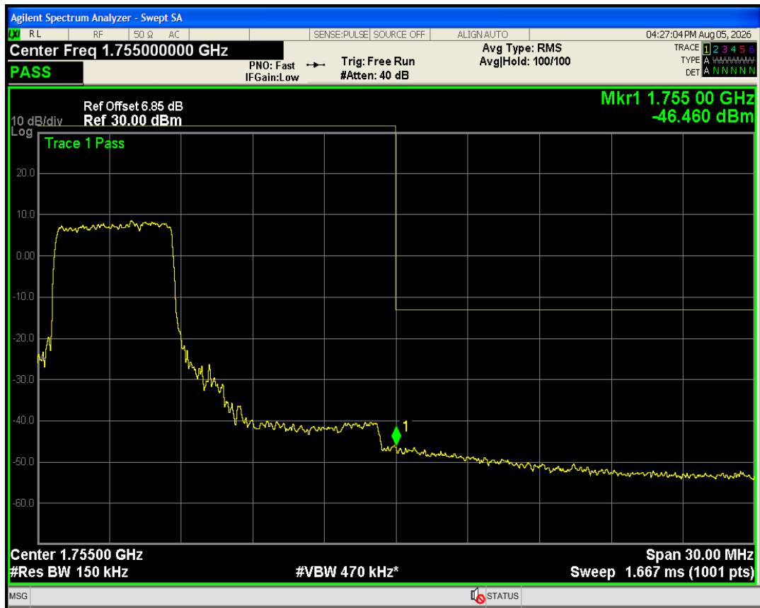
Band4 QAM16 BW=20MHz Channel=20050 RB Size=27 Position=#0
