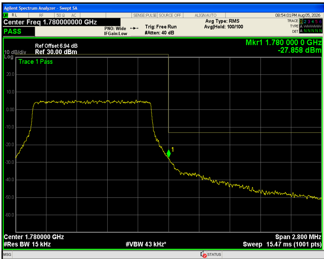
Band66 QPSK BW=1.4MHz Channel=132665 RB Size=6 Position=#0
