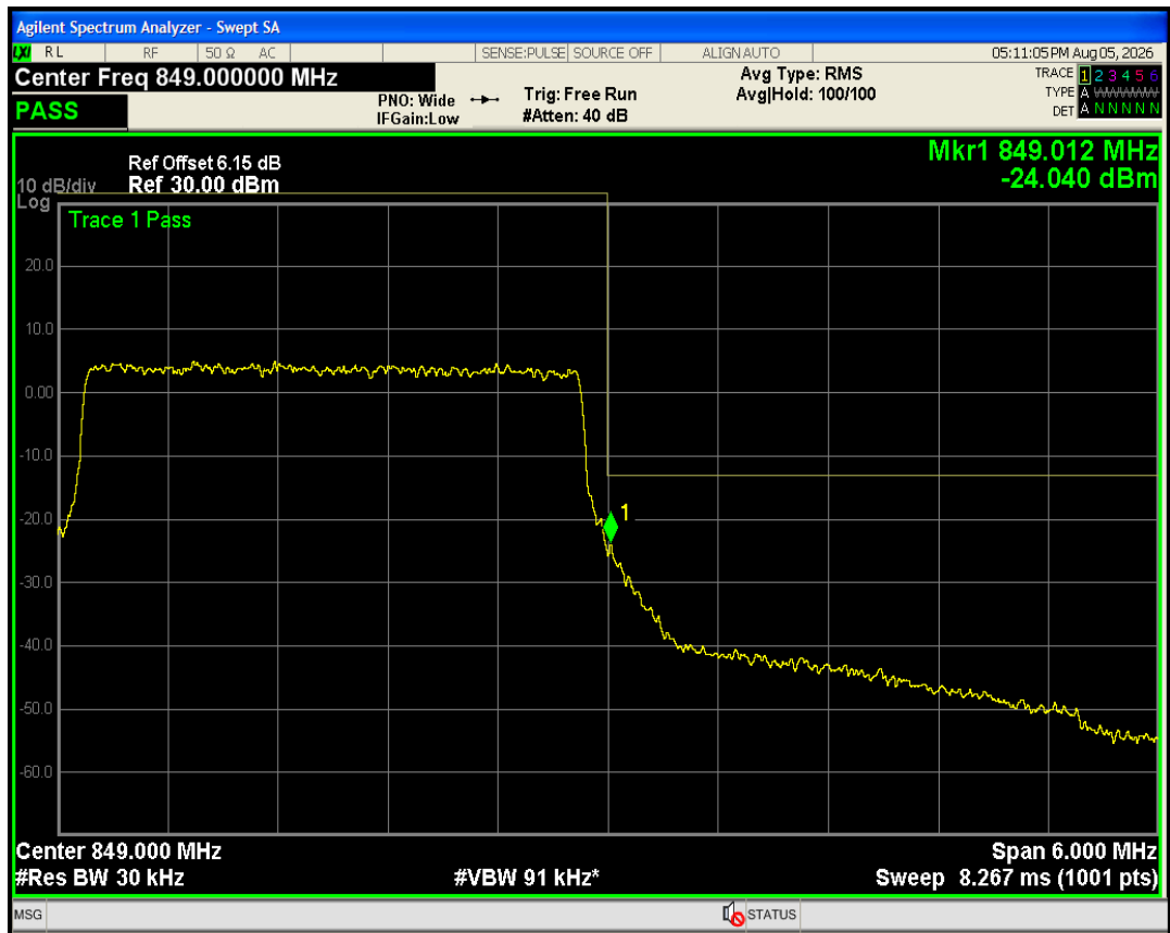
Band5 QPSK BW=5MHz Channel=20425 RB Size=25 Position=#0
