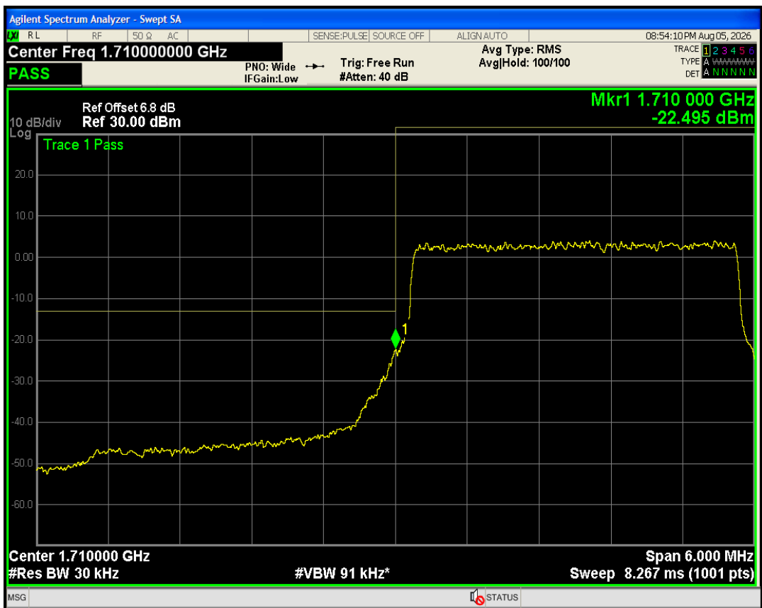
Band66 QPSK BW=3MHz Channel=132657 RB Size=15 Position=#0
