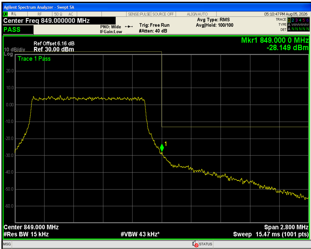
Band5 QPSK BW=3MHz Channel=20415 RB Size=15 Position=#0
