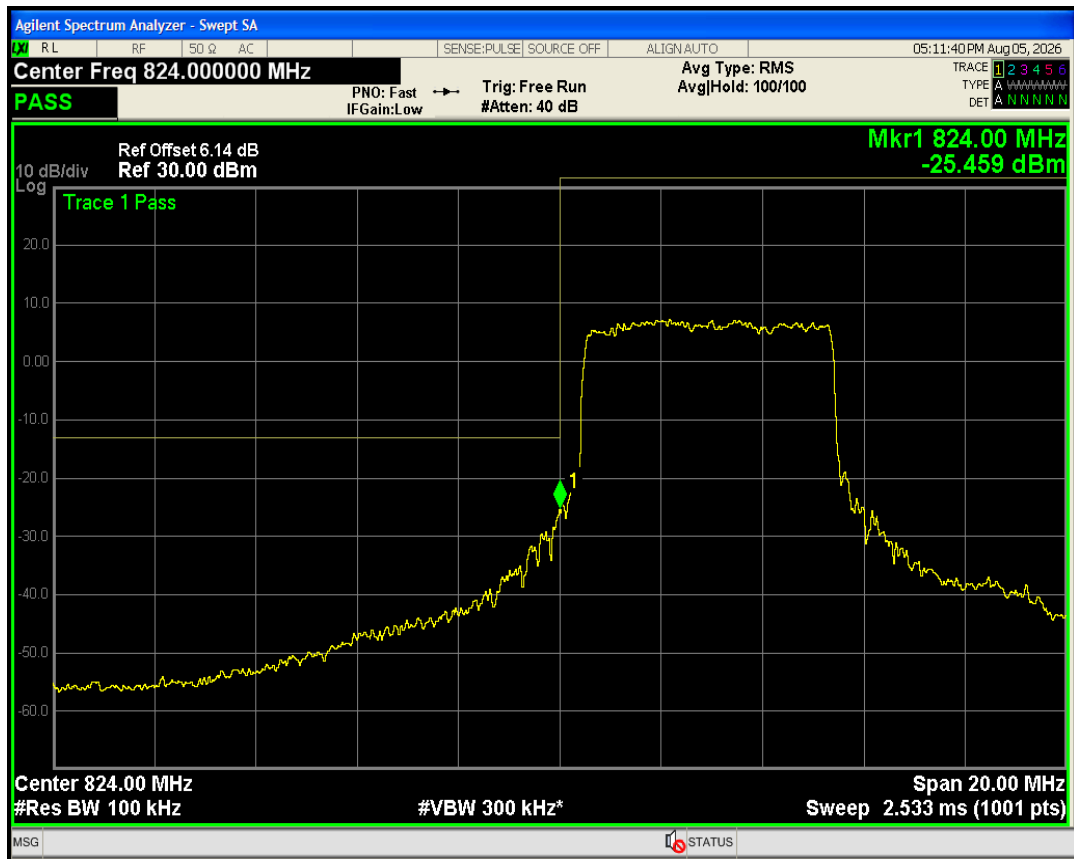
Band5 QPSK BW=10MHz Channel=20600 RB Size=50 Position=#0
