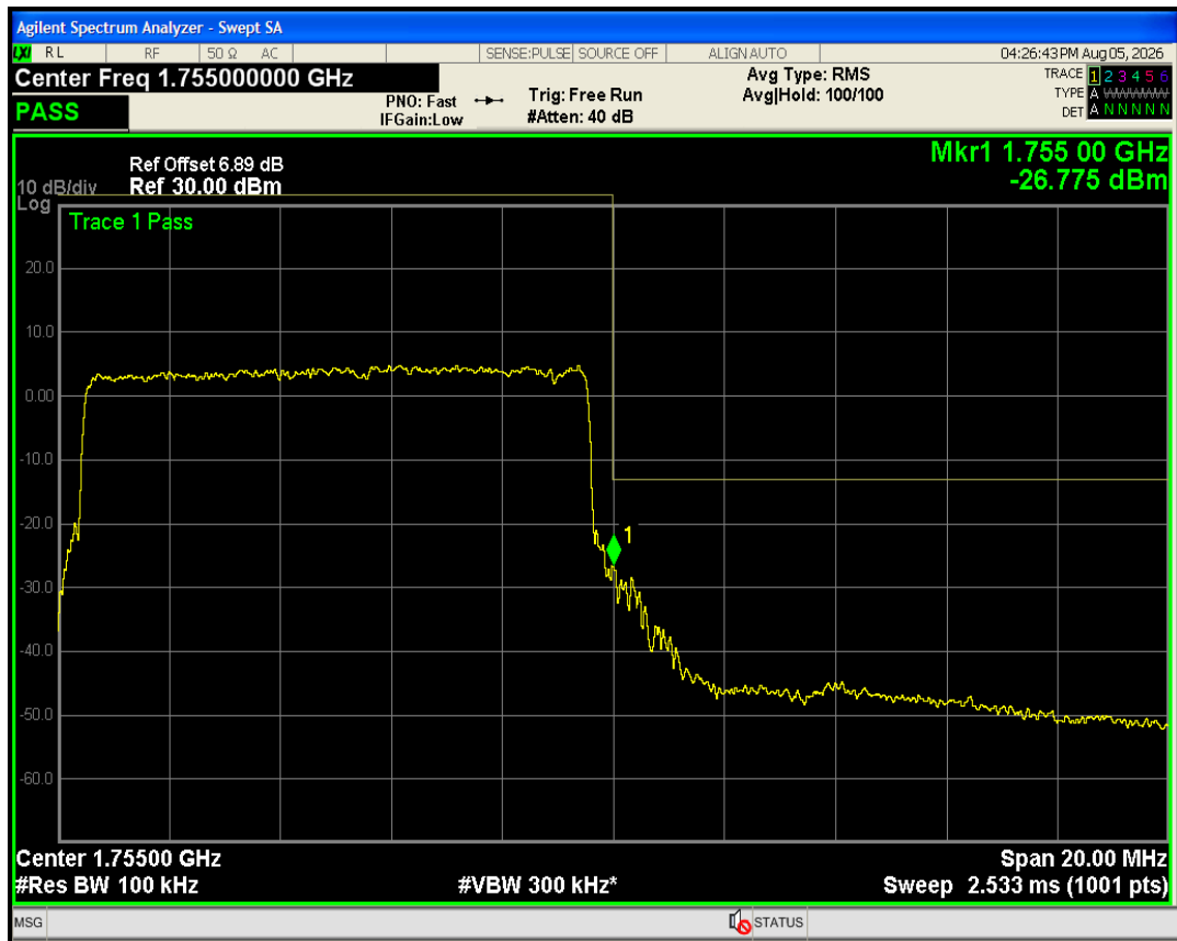
Band4 QAM16 BW=10MHz Channel=20000 RB Size=27 Position=#0
