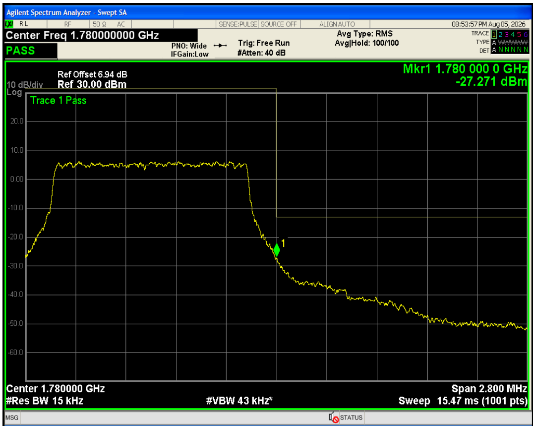
Band66 QPSK BW=3MHz Channel=131987 RB Size=15 Position=#0
