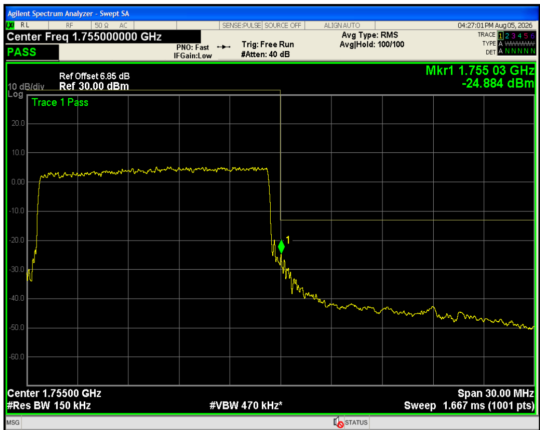
Band4 QAM16 BW=15MHz Channel=20325 RB Size=27 Position=#0
