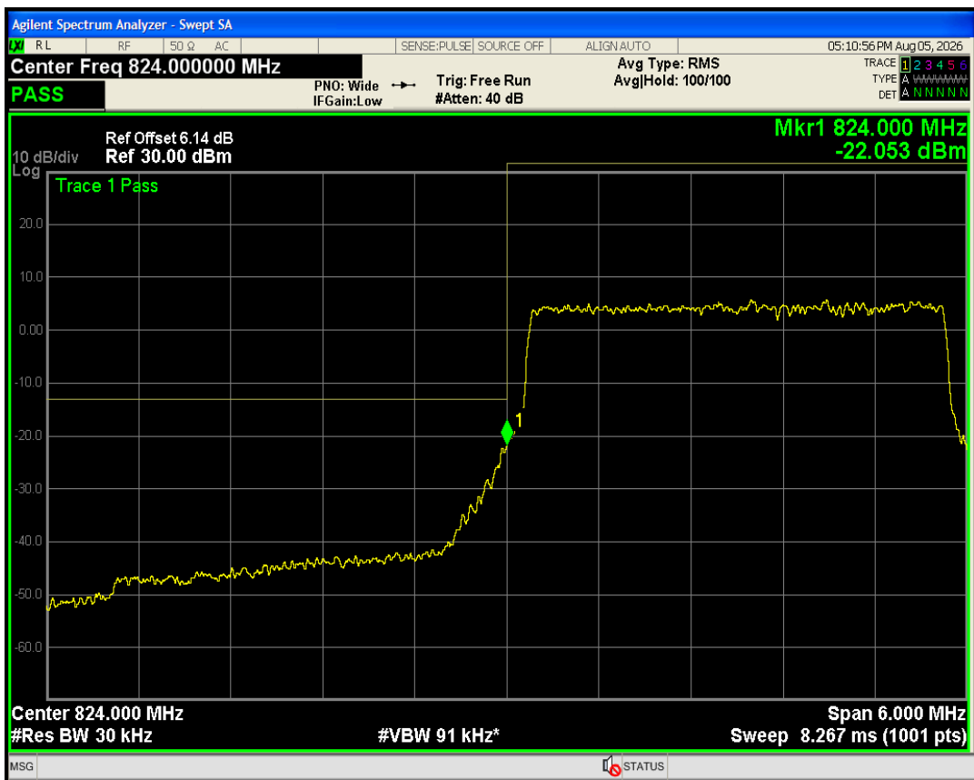
Band5 QAM16 BW=3MHz Channel=20415 RB Size=15 Position=#0
