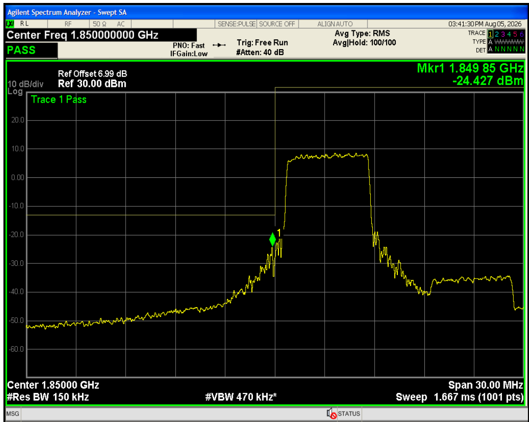
Band2 QAM16 BW=15MHz Channel=19125 RB Size=27 Position=#0
