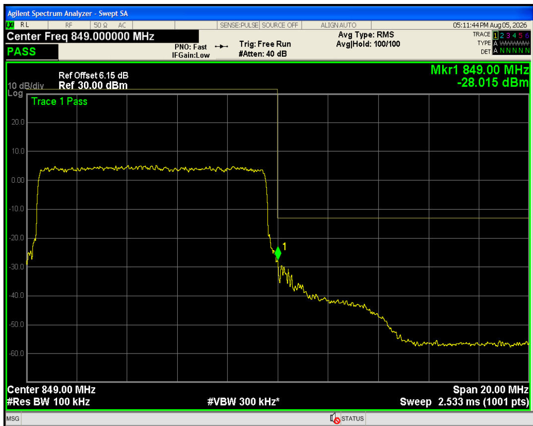
Band5 QAM16 BW=10MHz Channel=20600 RB Size=27 Position=#0
