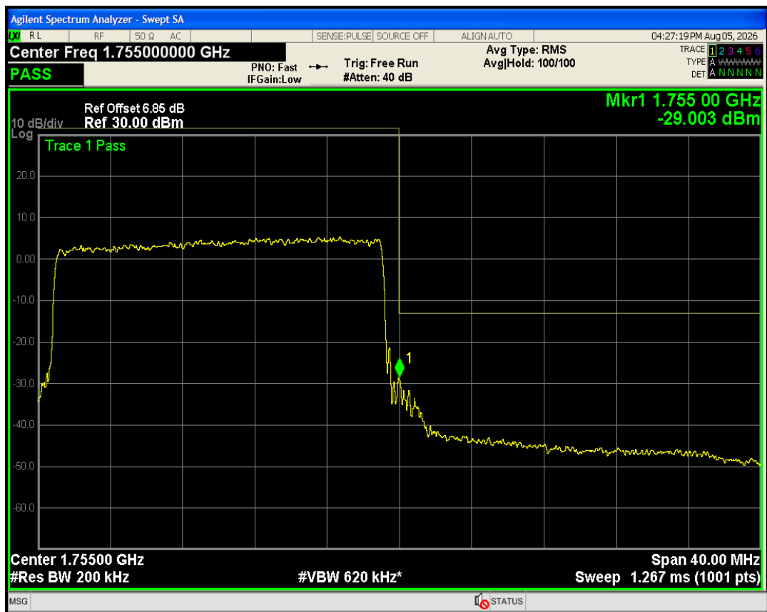
Band4 QAM16 BW=20MHz Channel=20300 RB Size=27 Position=#0
