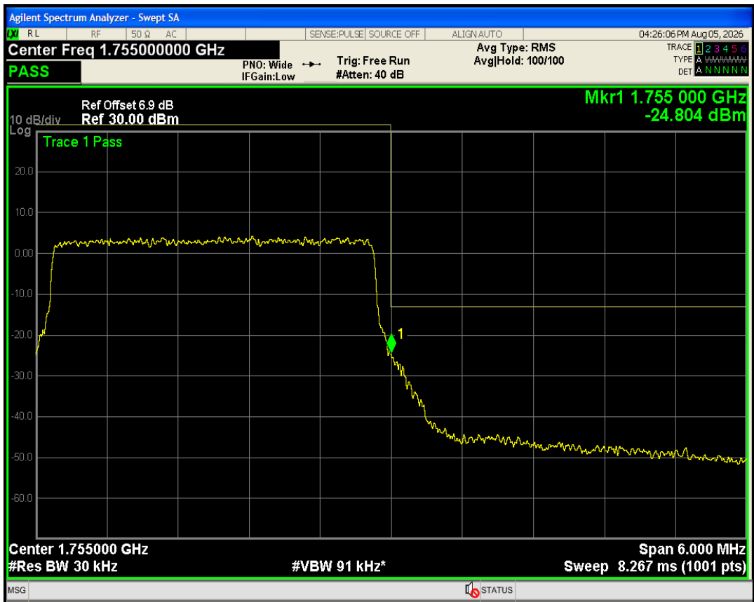
Band4 QPSK BW=5MHz Channel=19975 RB Size=25 Position=#0
