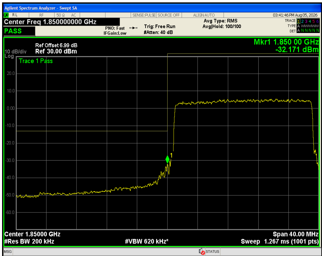
Band2 QAM16 BW=20MHz Channel=18700 RB Size=27 Position=#0
