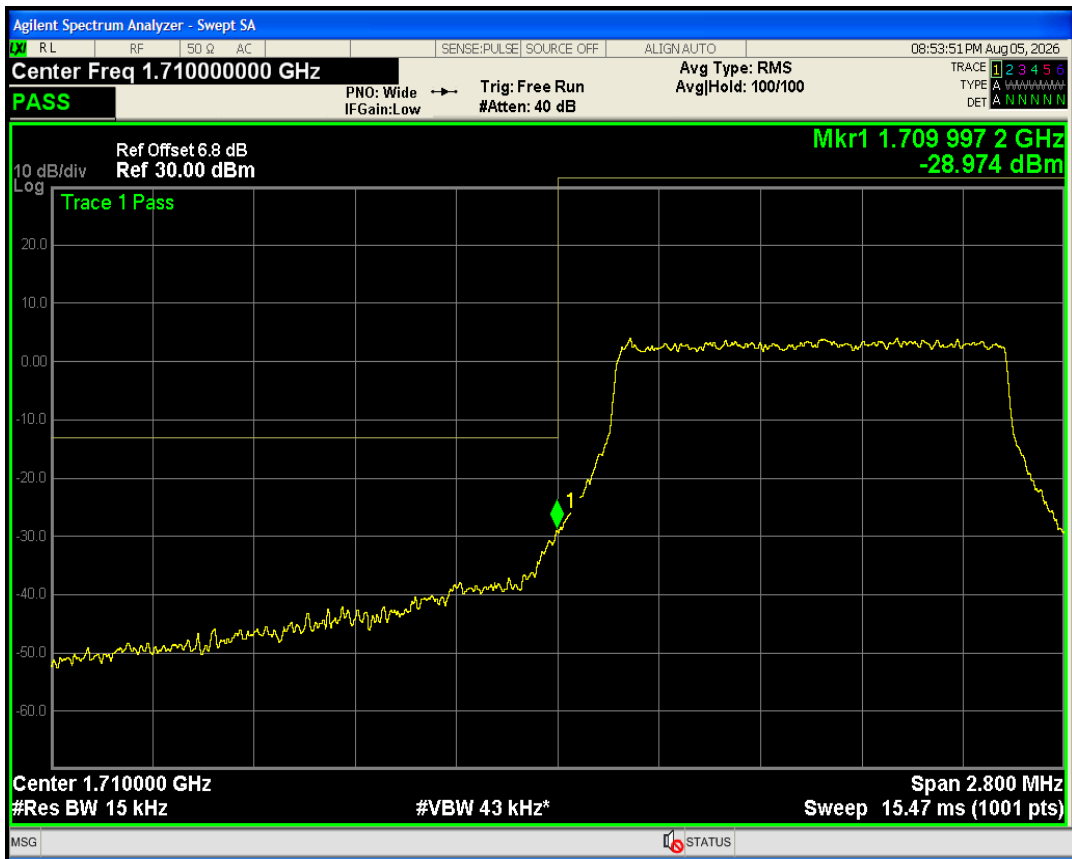
Band66 QAM16 BW=1.4MHz Channel=132665 RB Size=6 Position=#0
