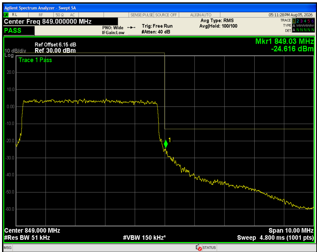
Band5 QPSK BW=5MHz Channel=20625 RB Size=25 Position=#0
