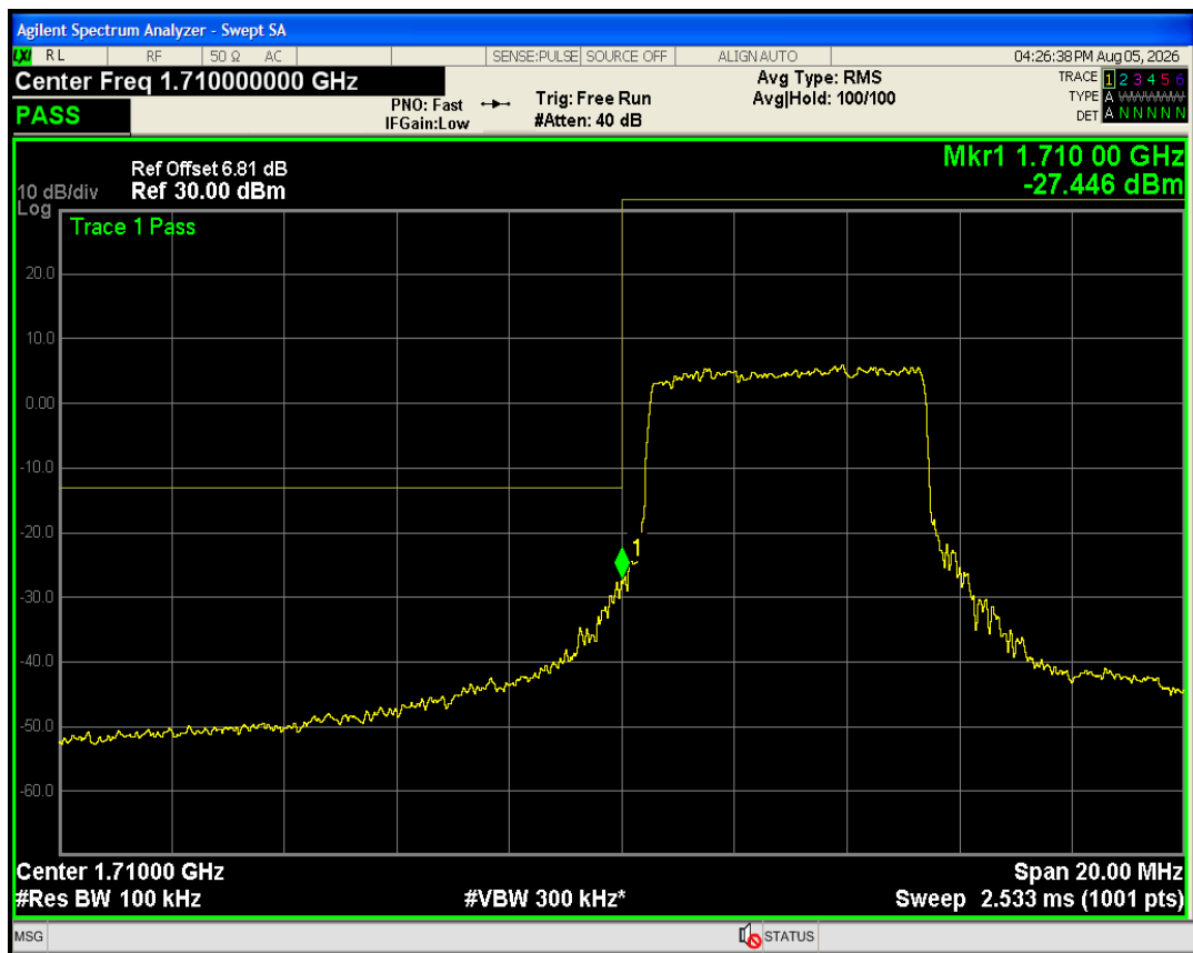
Band4 QAM16 BW=10MHz Channel=20350 RB Size=27 Position=#0
