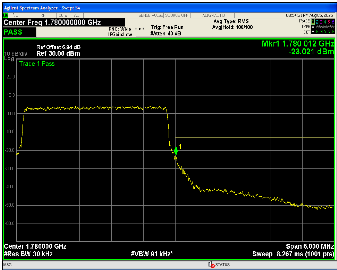
Band66 QPSK BW=5MHz Channel=131997 RB Size=25 Position=#0
