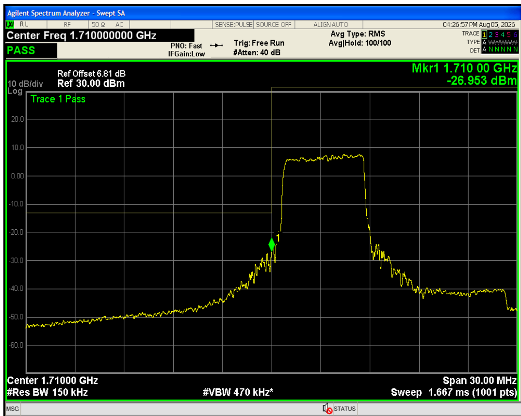
Band4 QPSK BW=15MHz Channel=20025 RB Size=75 Position=#0
