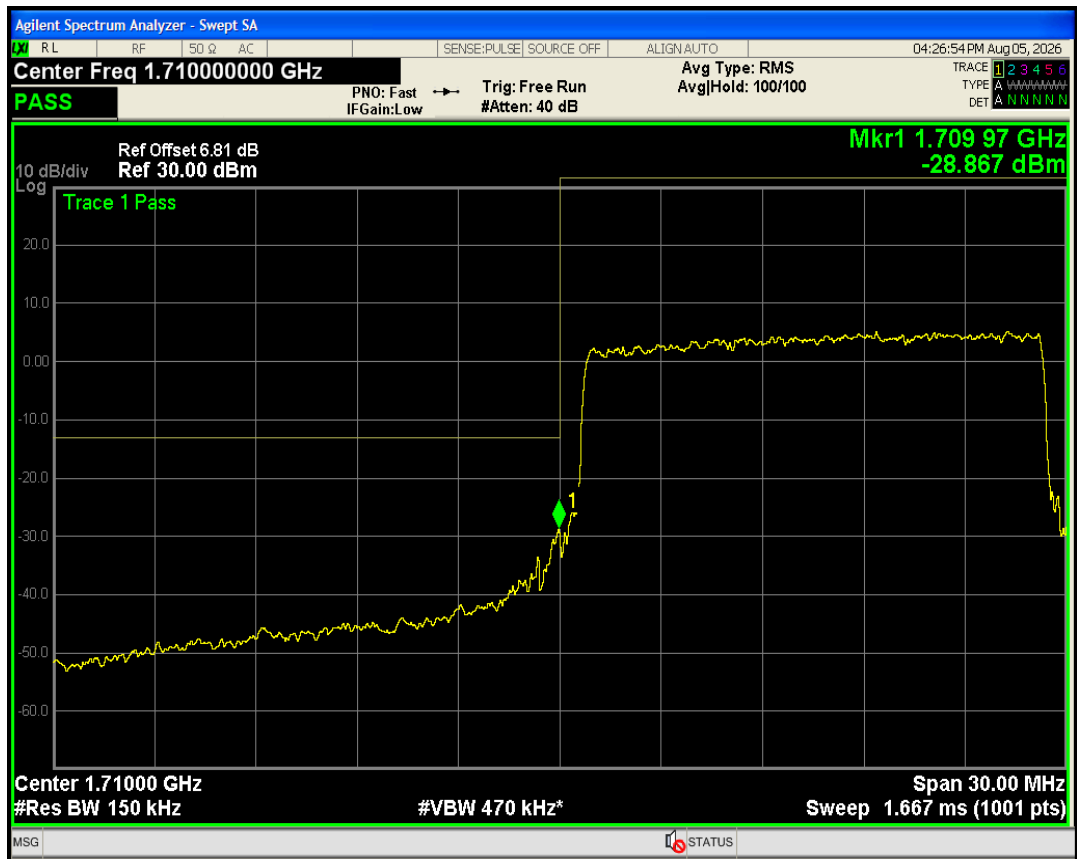
Band4 QPSK BW=15MHz Channel=20325 RB Size=75 Position=#0
