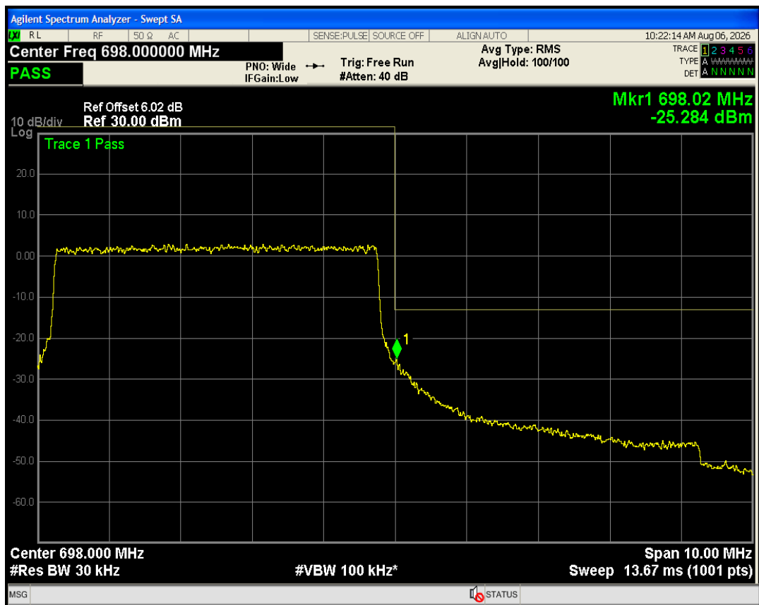
Band71 QAM16 BW=5MHz Channel=133447 RB Size=25 Position=#0
