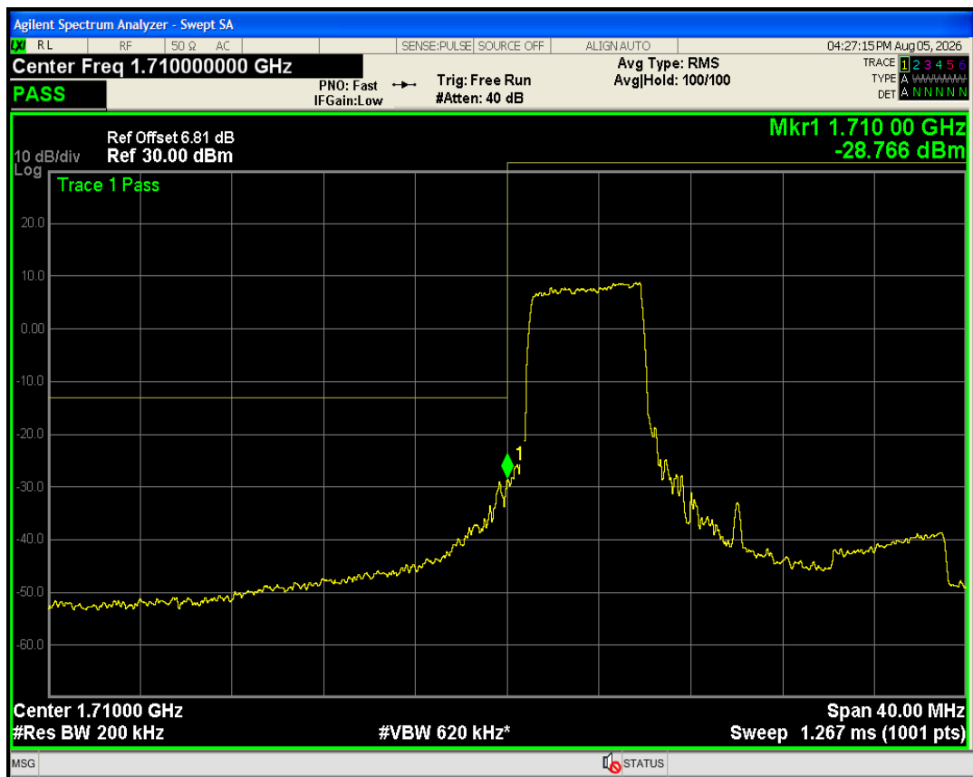
Band4 QPSK BW=20MHz Channel=20050 RB Size=100 Position=#0
