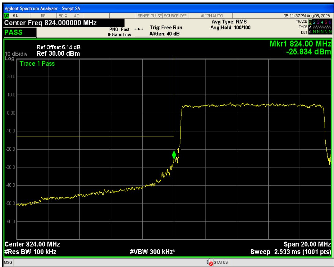
Band5 QAM16 BW=10MHz Channel=20450 RB Size=27 Position=#0
