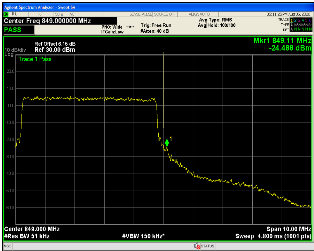
Band5 QPSK BW=10MHz Channel=20450 RB Size=50 Position=#0
