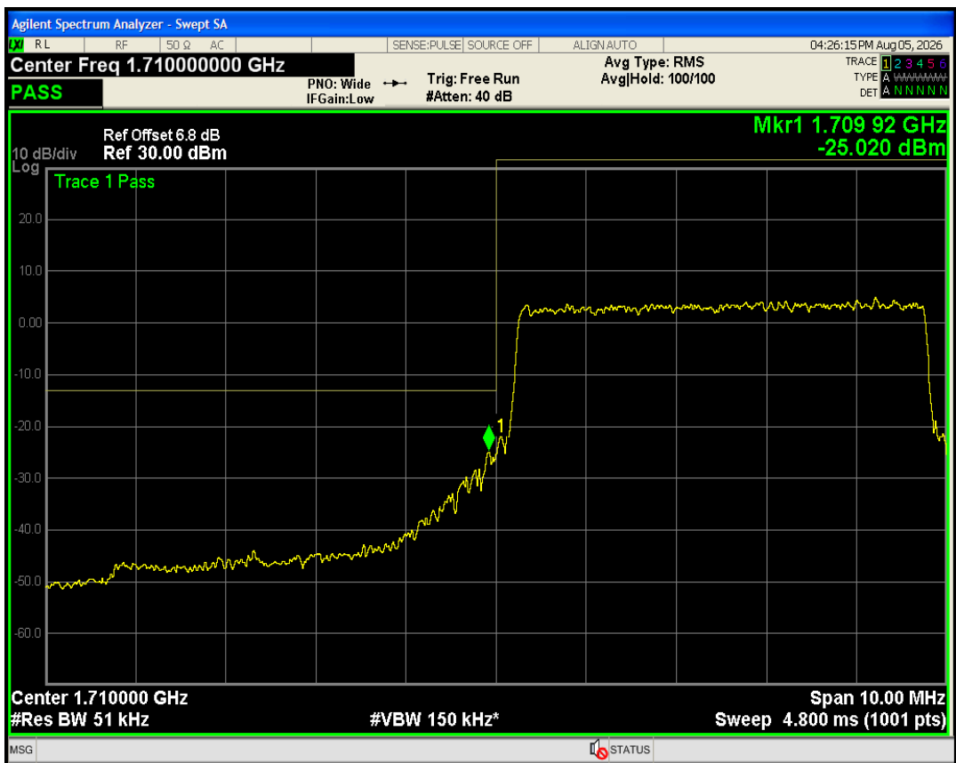
Band4 QAM16 BW=5MHz Channel=19975 RB Size=25 Position=#0
