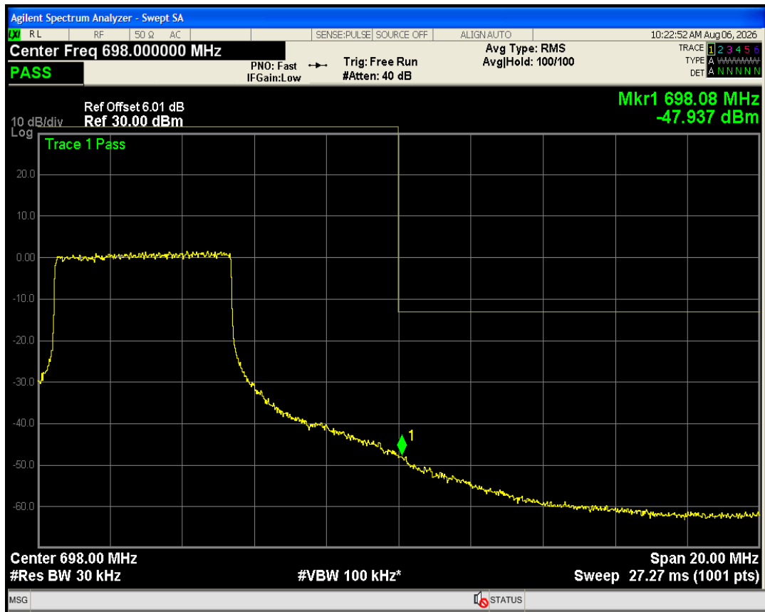
Band71 QPSK BW=15MHz Channel=133197 RB Size=75 Position=#0
