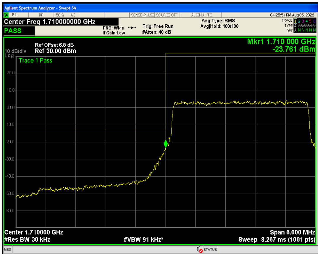
Band4 QAM16 BW=3MHz Channel=19965 RB Size=15 Position=#0
