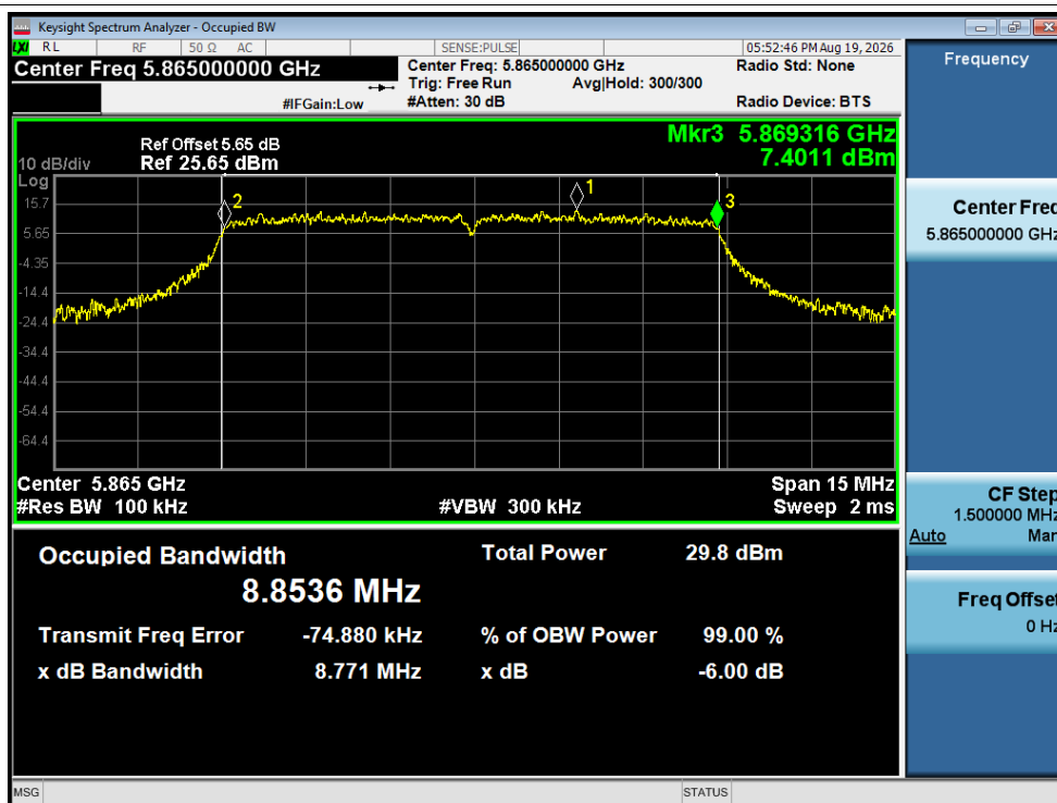
-6dB Bandwidth NVNT 10M 5865MHz Ant2
