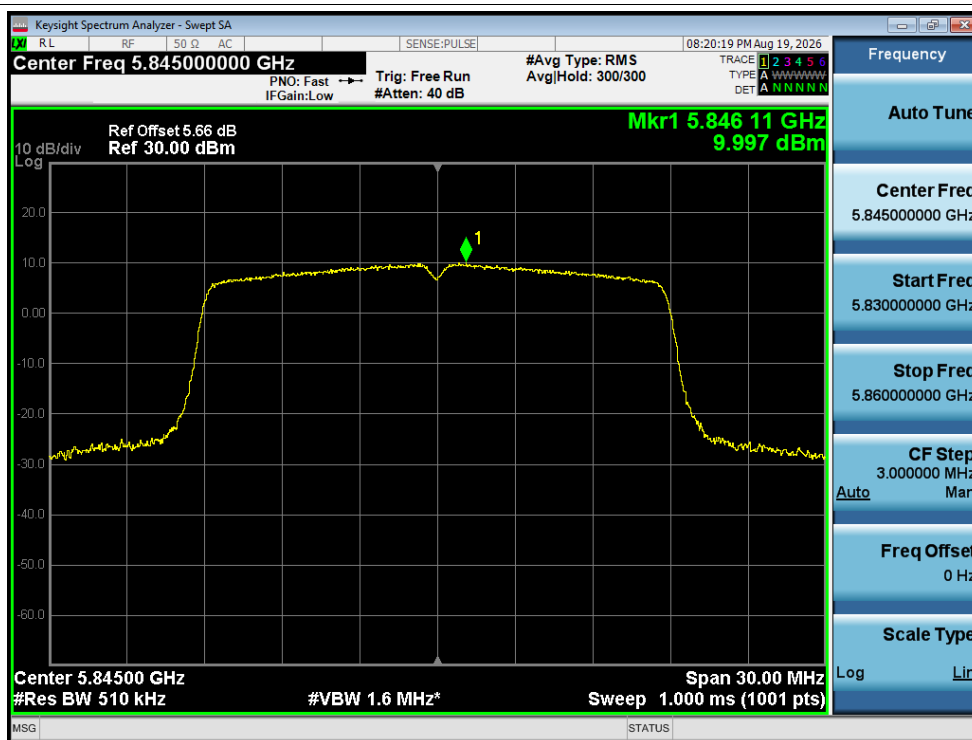
PSD NVNT 20M 5845MHz Ant2
