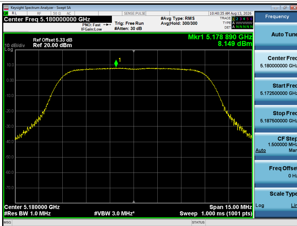
PSD NVNT 10M 5180MHz Ant2
