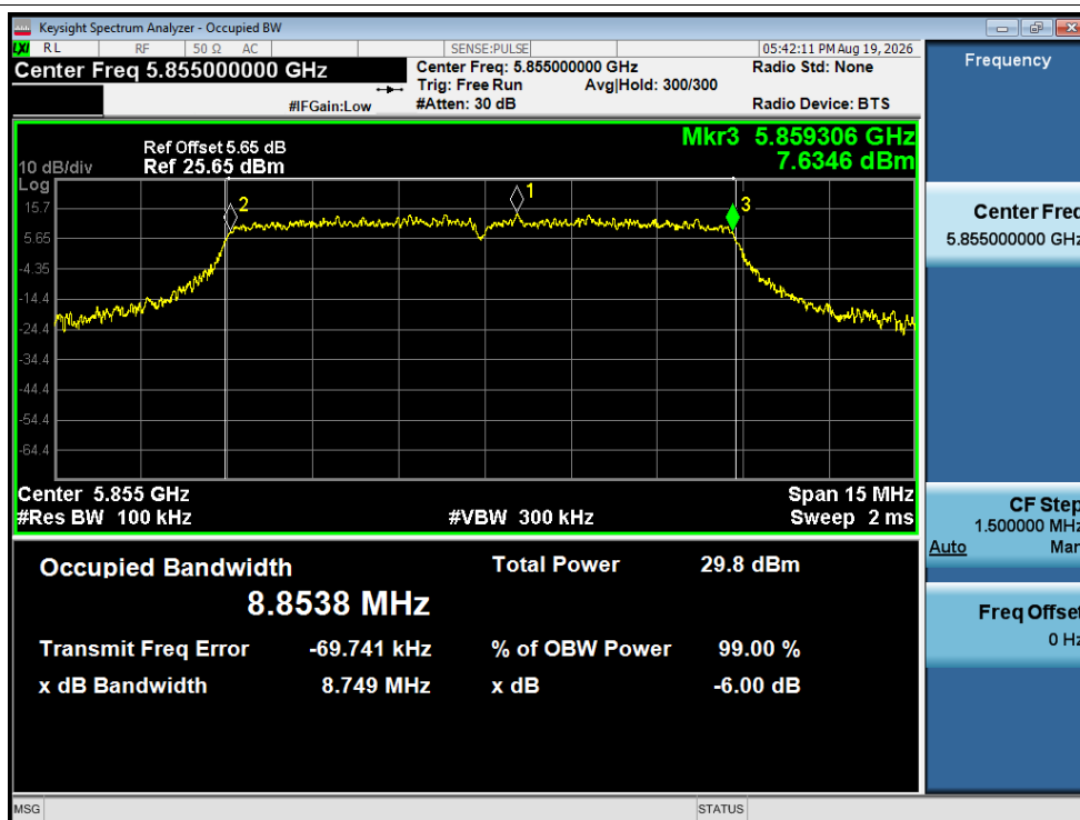
-6dB Bandwidth NVNT 10M 5855MHz Ant2
