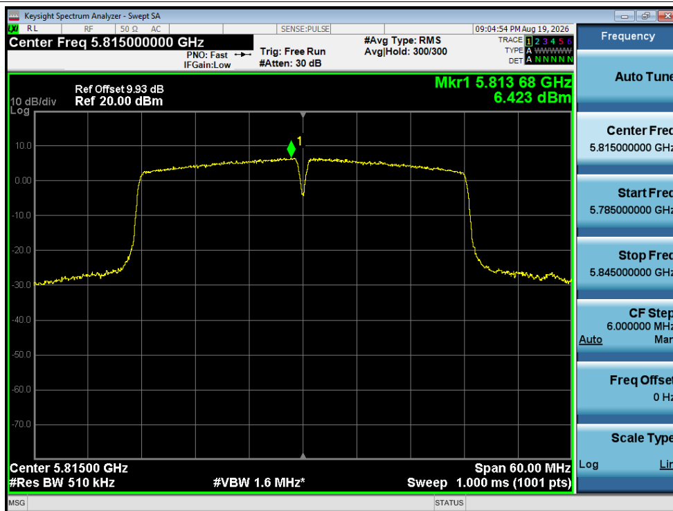
PSD NVNT 40M 5815MHz Ant1
