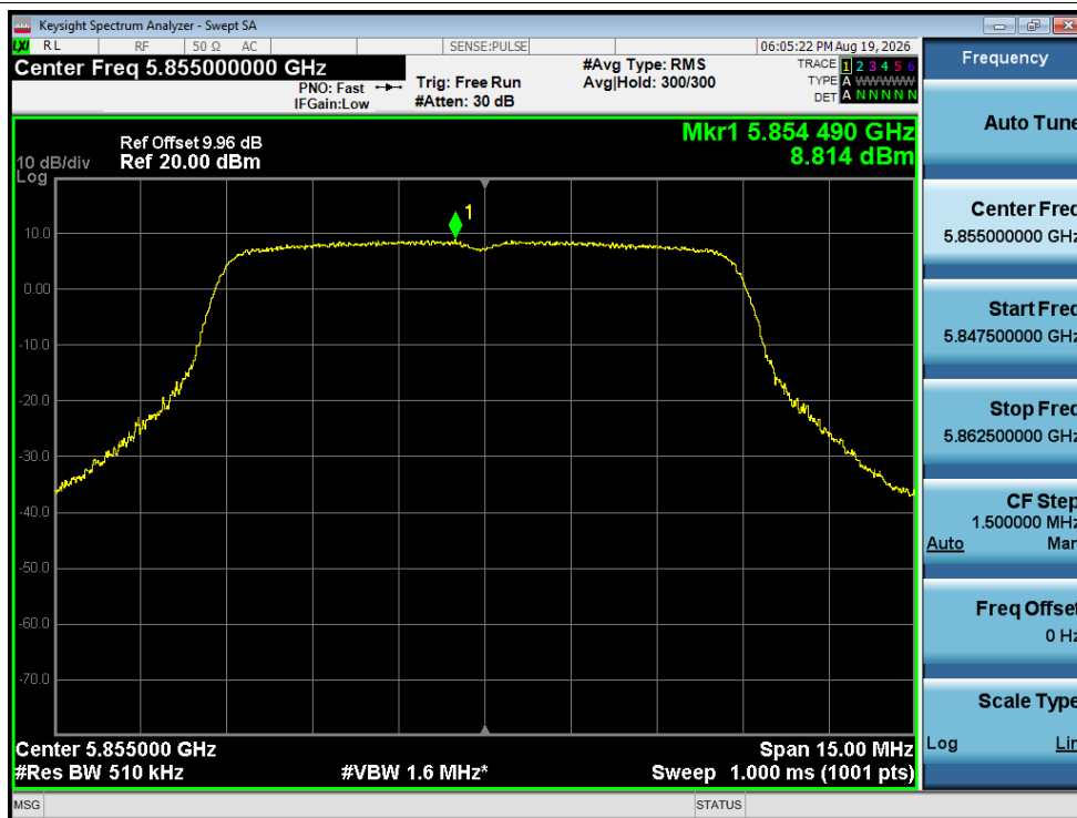
PSD NVNT 10M 5855MHz Ant1
