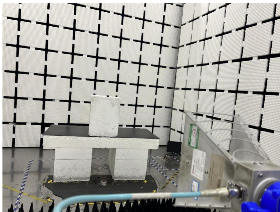
Radiation Emission Test Setup (1GHz to 18GHz)
