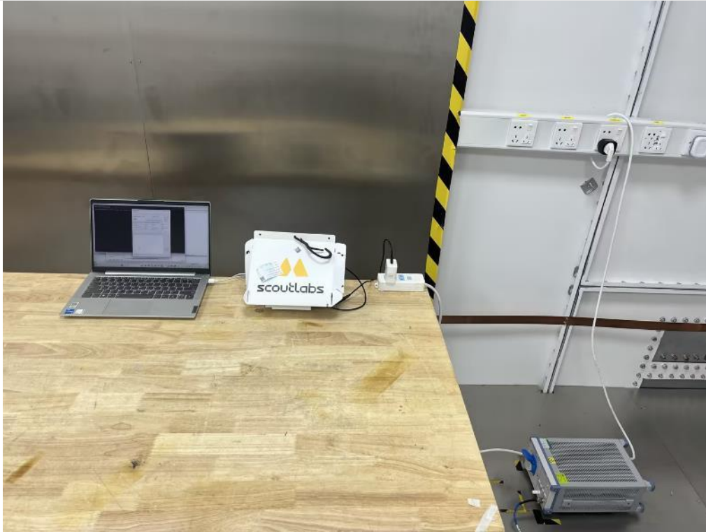
AC Power Line Conducted Emission
