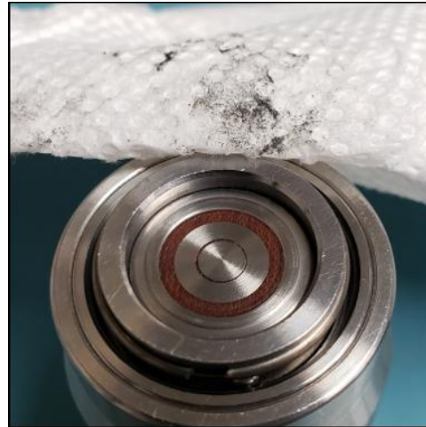
Probe sensor face visually clean using a clean lint-free dry cotton cloth
