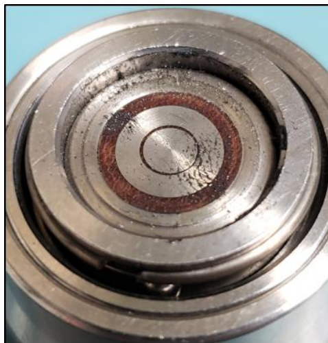
Dirty or contaminated probe sensor face
