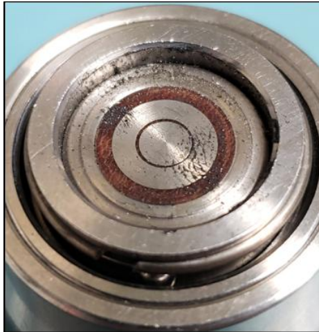
Dirty or contaminated probe sensor face
