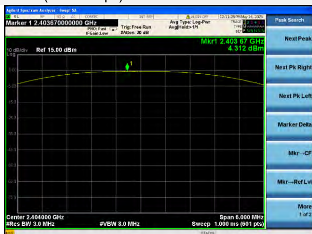
GFSK (BLE 2Mbps) LOW CHANNEL
