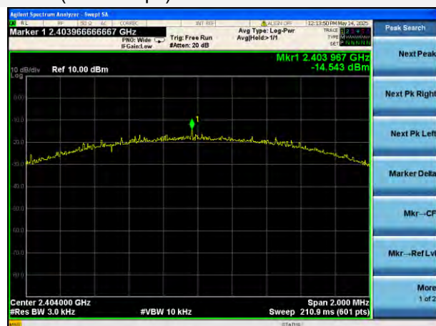
GFSK (BLE 2Mbps) LOW CHANNEL
