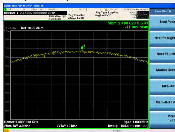
GFSK (BLE 1Mbps) HIGH CHANNEL
