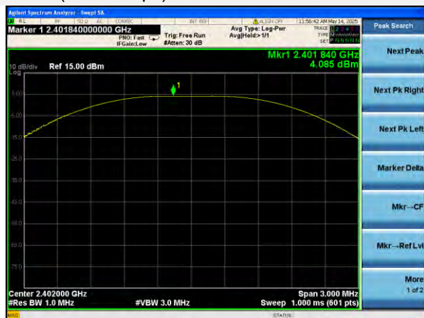
GFSK (BLE 1Mbps) LOW CHANNEL
