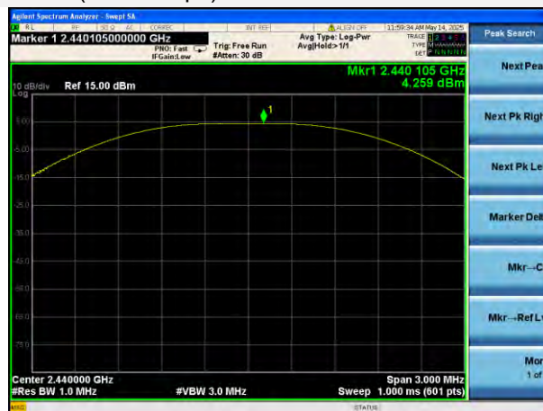
GFSK (BLE 1Mbps) MIDDLE CHANNEL
