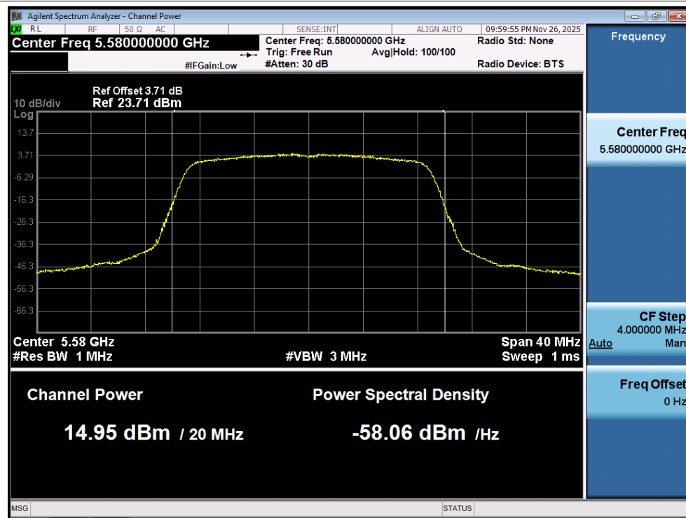
Power NVNT ac20 5580MHz Ant1
