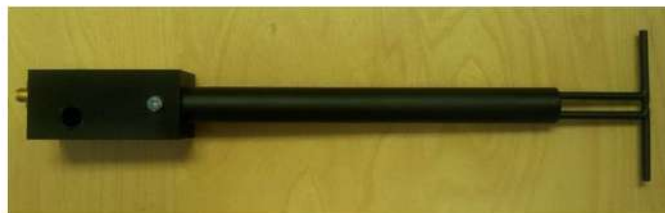
Figure 1 – MVG COMOSAR Validation Dipole
