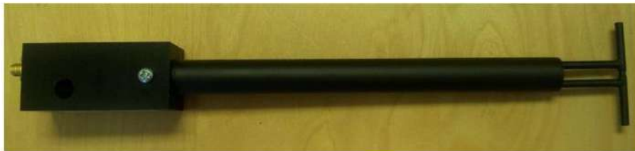
Figure 1 – MVG COMOSAR Validation Dipole
