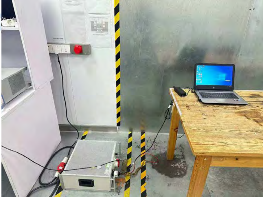
Conducted Emission at AC power line
