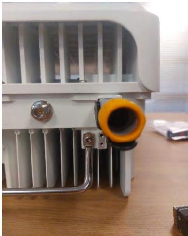
14 – Main Label Main label will be going on the lower half of the right handside of the unit (opposite to air vent)
