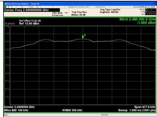
In-Band Reference Level BLE 1M_Channel 39
