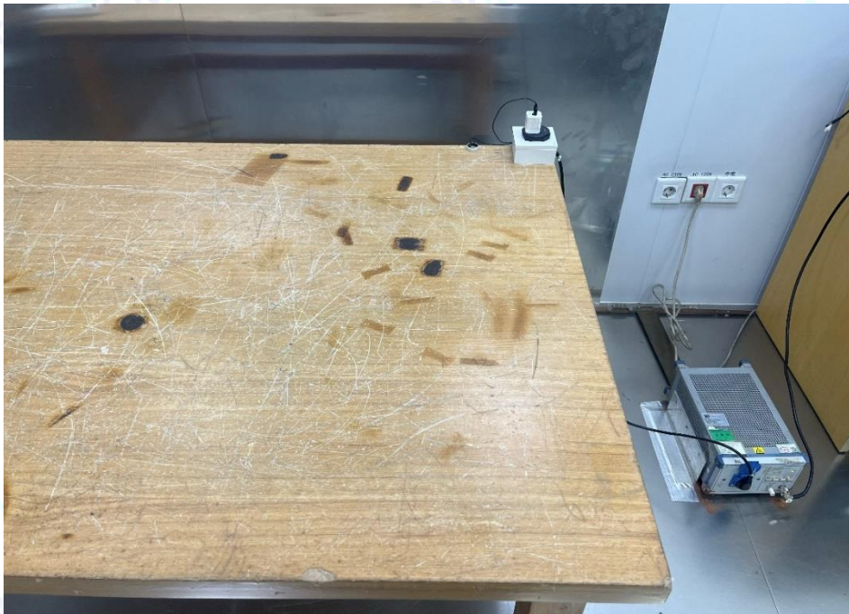
Photo of Setup for Radiated Emission (30MHz~1GHz)
