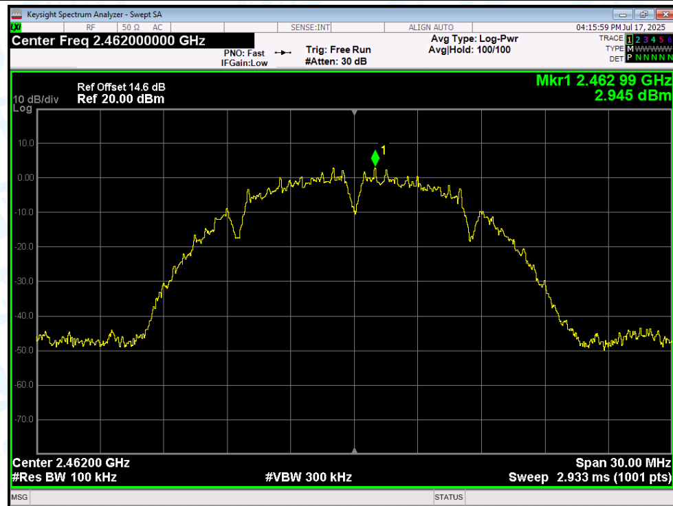
Band Edge NVNT b 2462MHz Ant1 Emission
