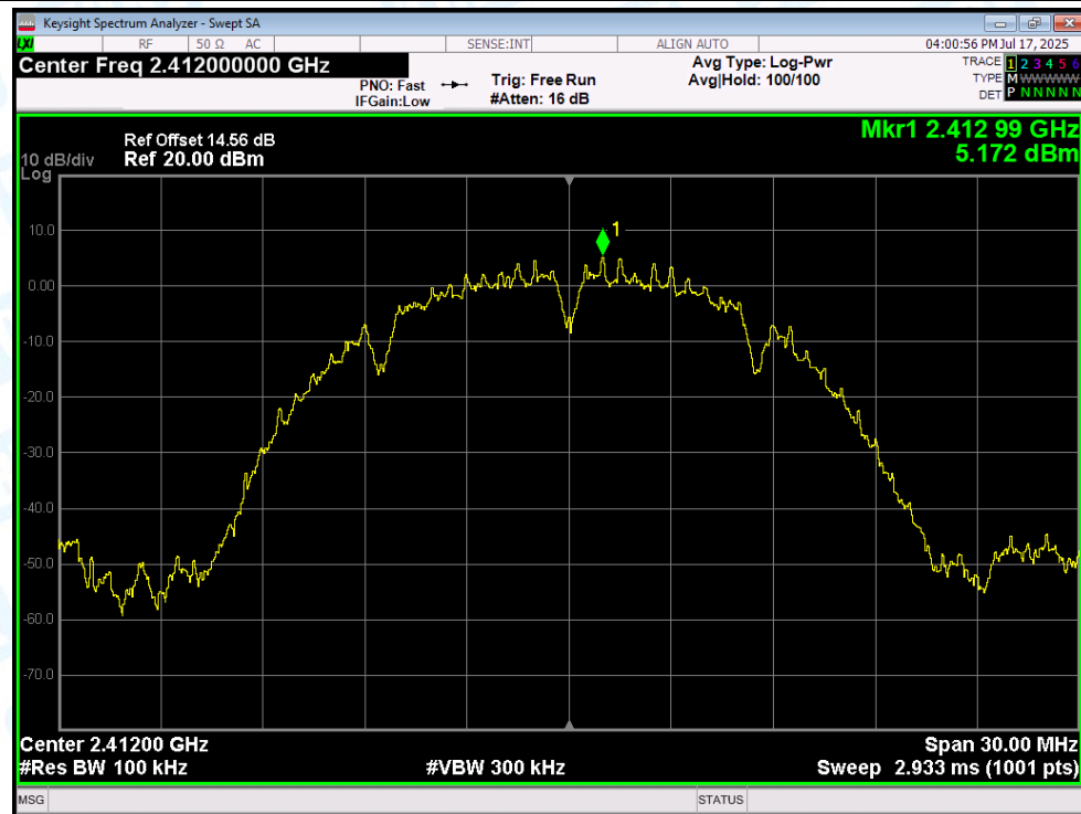
Tx. Spurious NVNT b 2412MHz Ant1 Emission
