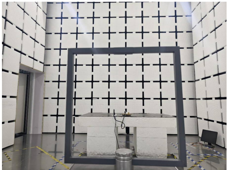
Radiation Emission Test Setup (Below 30MHz)
