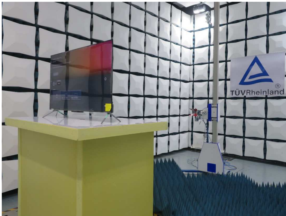
Photograph 7: Set-up photo for Radiated Spurious Emission, 1GHz - 18GHz
