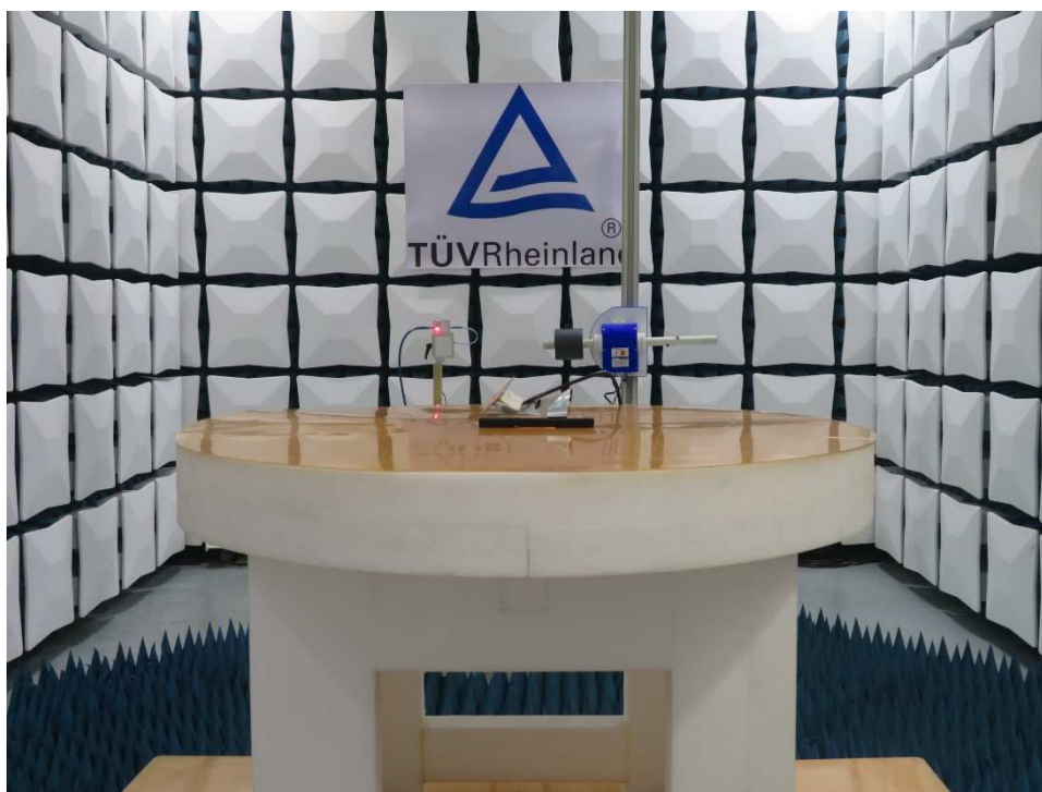
Photograph 3: Set-up photo for Radiated Spurious Emission, 18GHz - 40GHz
