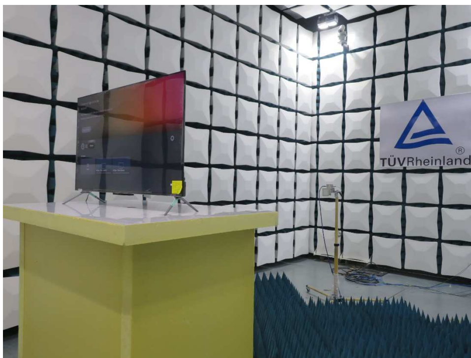
Photograph 8: Set-up photo for Radiated Spurious Emission, 18GHz - 40GHz
