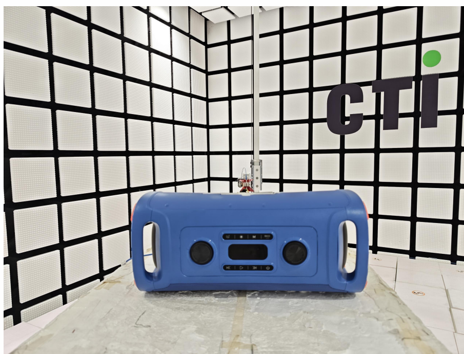
Radiated spurious emission Test Setup-2(Above 1GHz)
