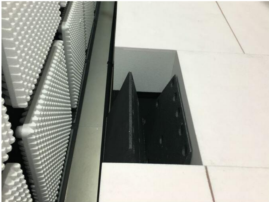
Radiated spurious emission Test Setup-6 There are absorbing materials under the ground.
