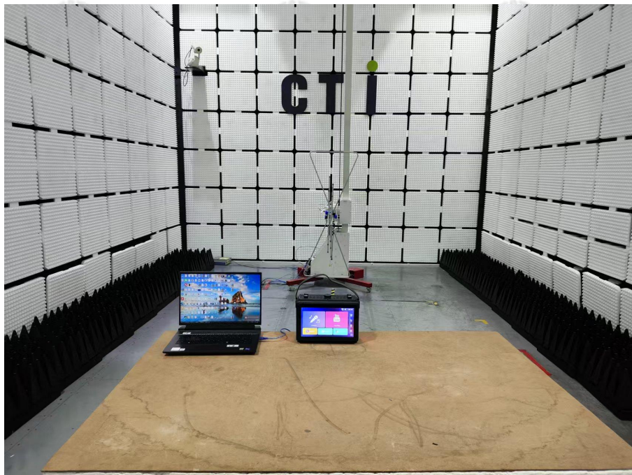
Radiated spurious emission Test Setup-1(Below 1GHz)
