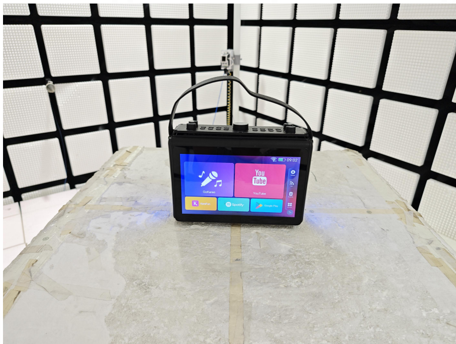
Radiated spurious emission Test Setup-3(Above 18GHz)
