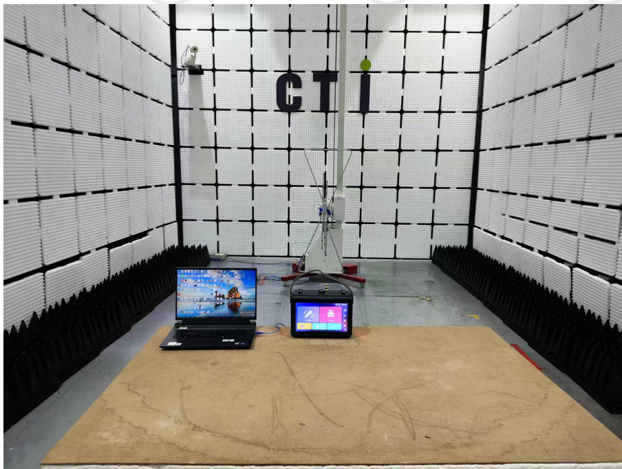
Radiated spurious emission Test Setup-1(Below 1GHz)
