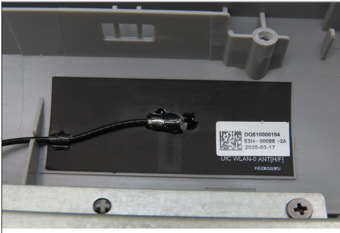
BT Antenna (Brand: Advanced Wireless & Antenna INC. / Model: ABF8P-100000A)
