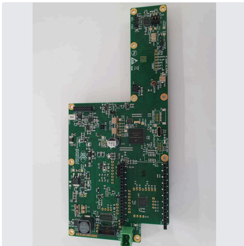
Photo 11 Oscillator and Modulator Board top
