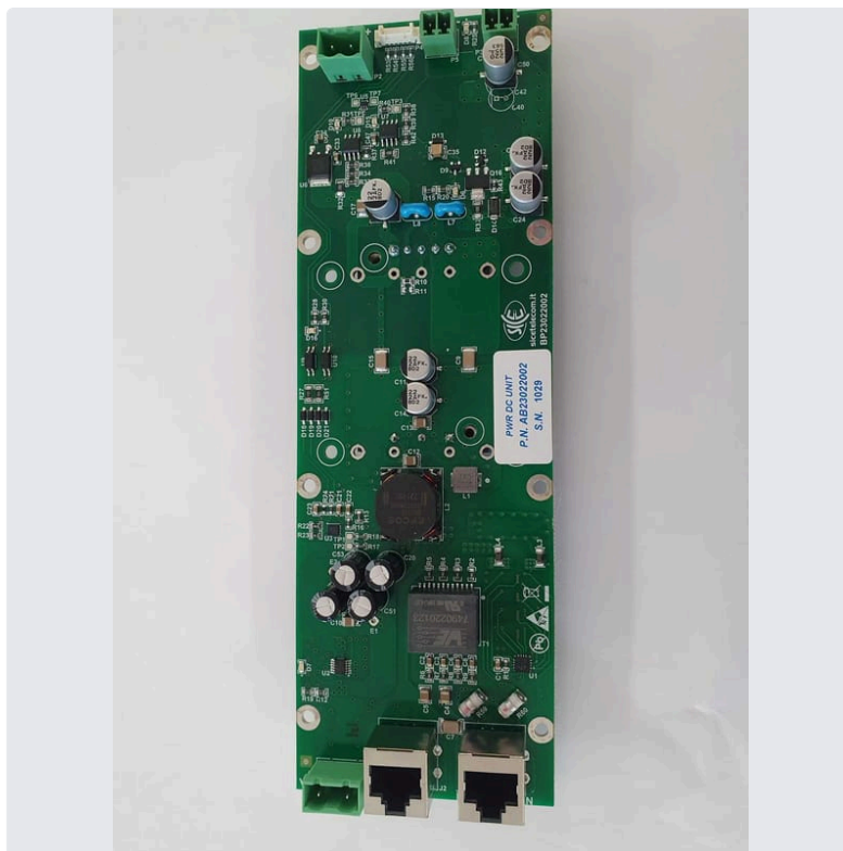
Photo 15 Power Supply Board top
