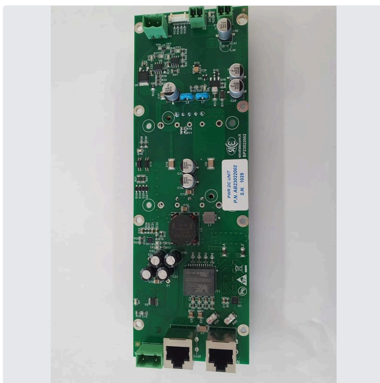
Photo 12 Power Supply Board top
