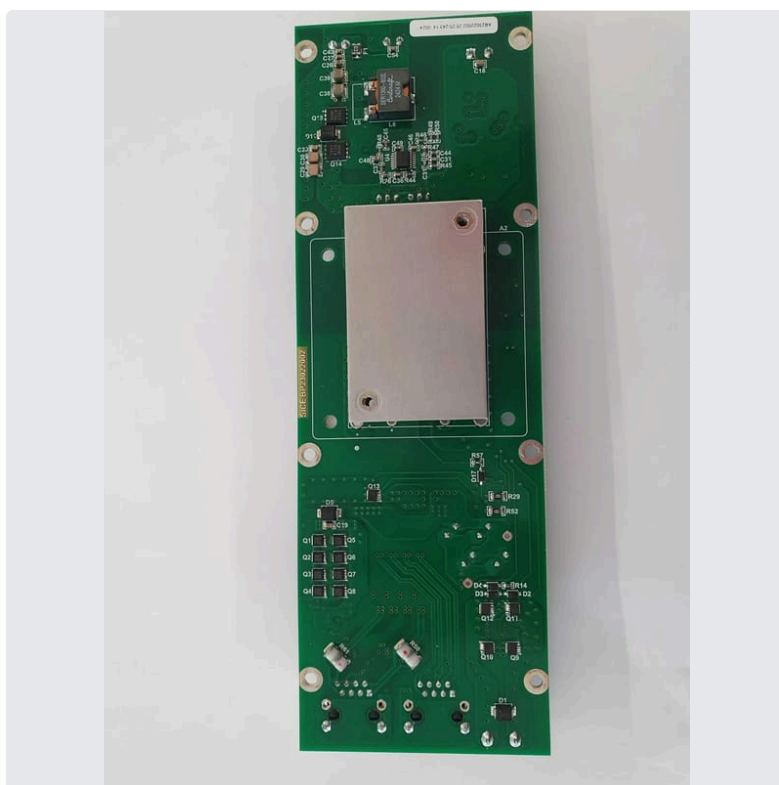
Photo 11 Power Supply Board bottom
