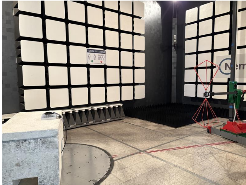
Figure 3.5-3: EUT Set-up photo for Radiated Emissions [30 MHz to 200 MHz]
