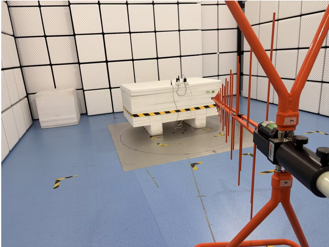
Radiation Emission - Back View (Below 1GHz)
