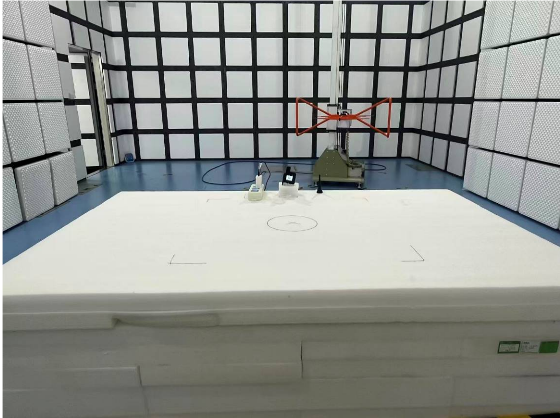
Radiation Emission - Back View (Below 1GHz)
