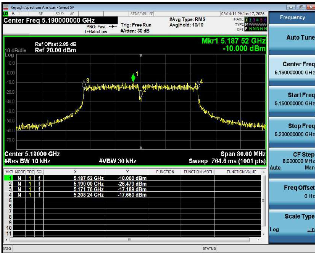
Freq. Stability NVNT n40 5190MHz Ant1
