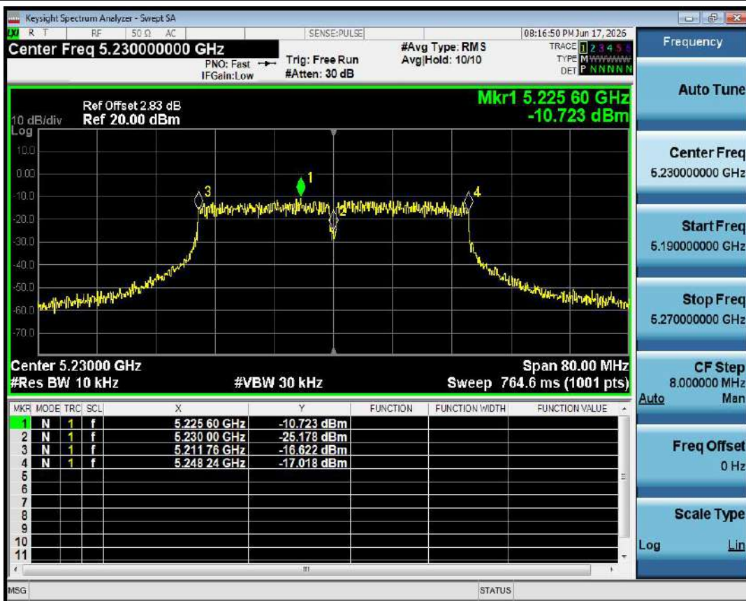
Freq. Stability NVNT n40 5230MHz Ant1
