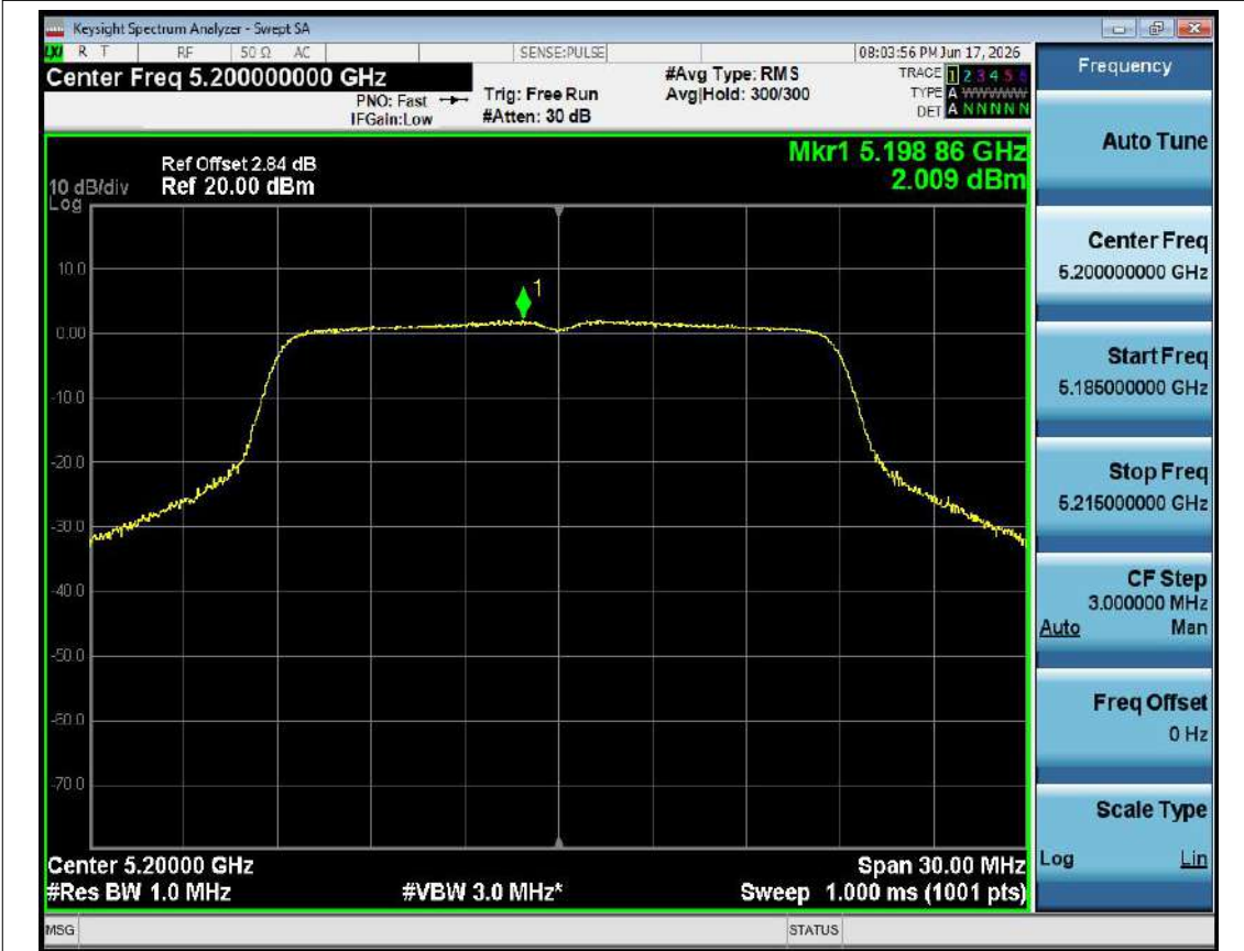
PSD NVNT ac20 5200MHz Ant1
