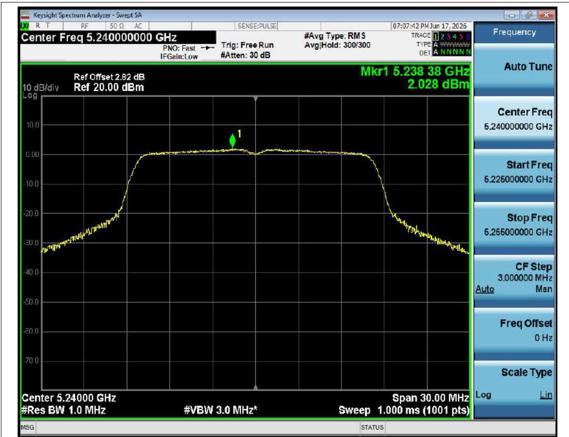
PSD NVNT a 5240MHz Ant1
