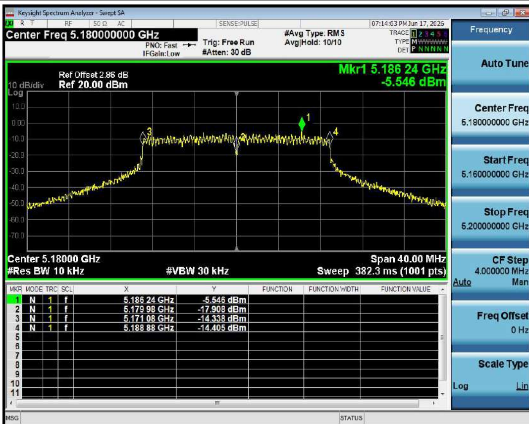
Freq. Stability NVNT n20 5180MHz Ant1
