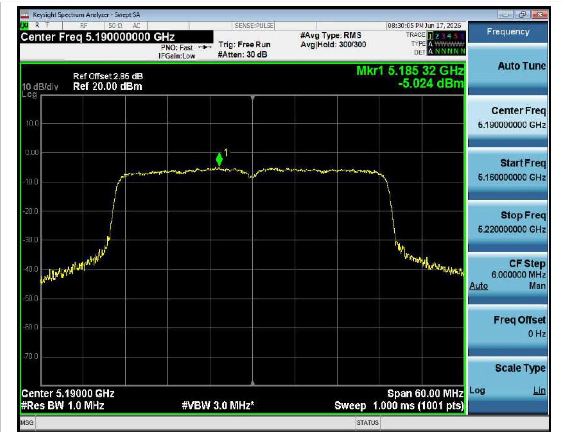
PSD NVNT ax40 5190MHz Ant1
