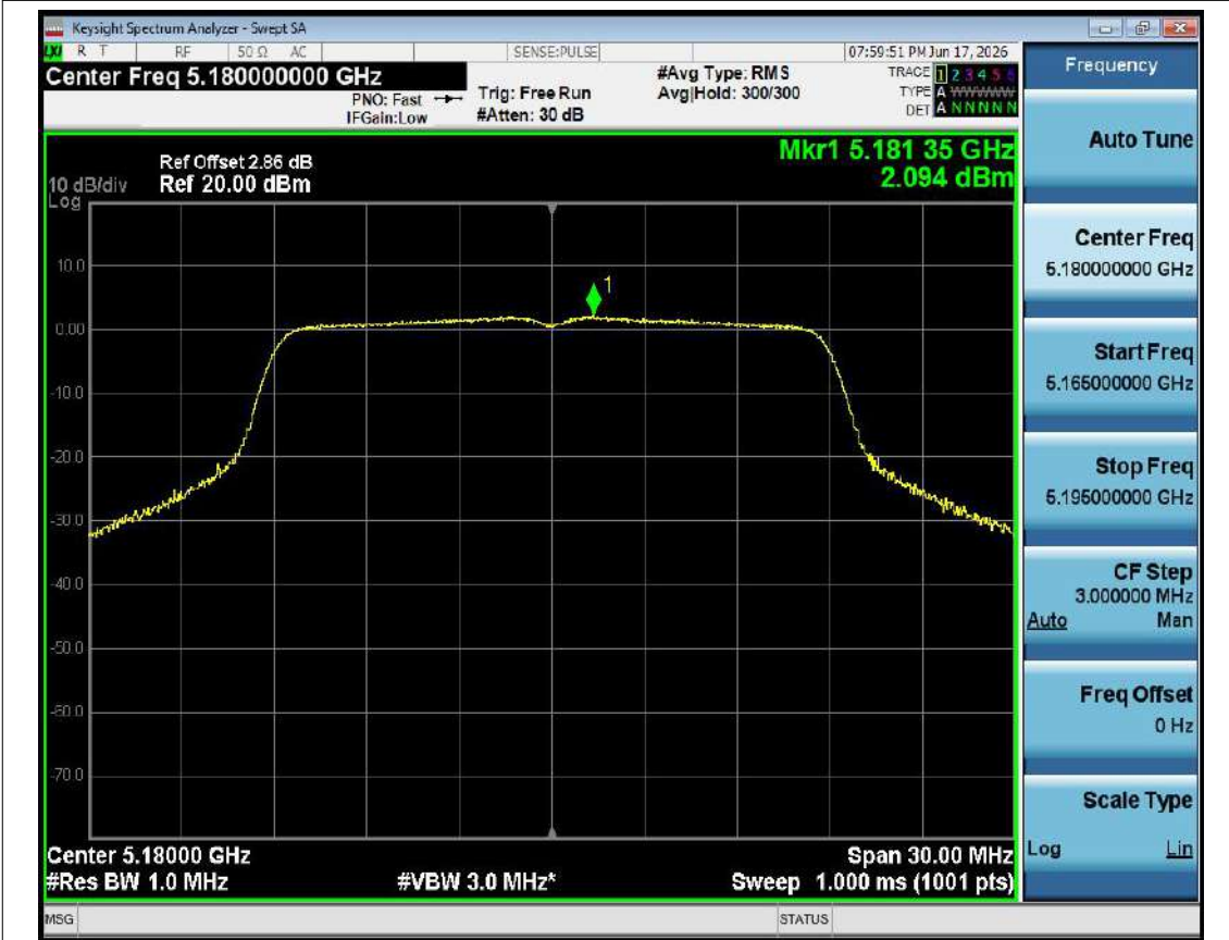
PSD NVNT n20 5180MHz Ant1
