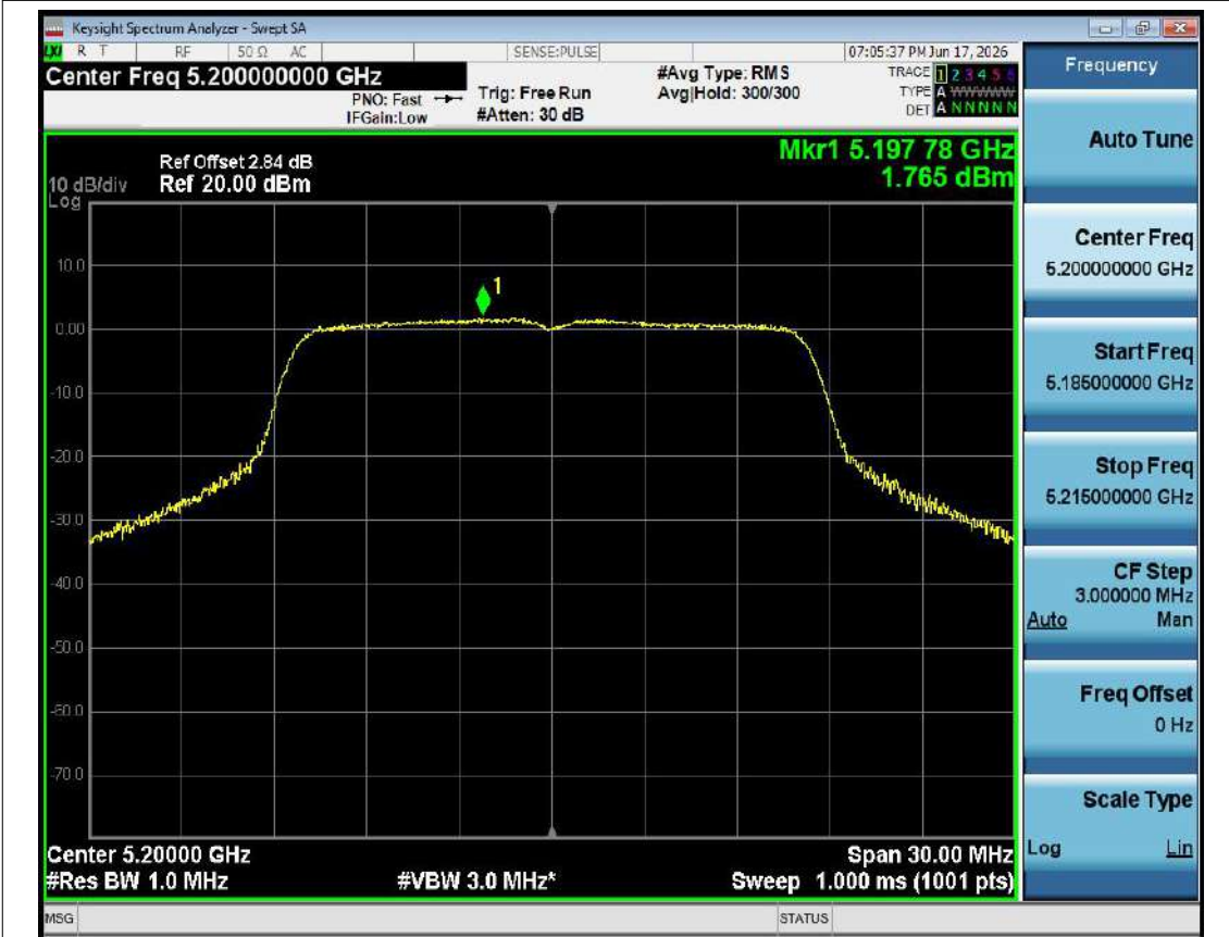
PSD NVNT a 5200MHz Ant1
