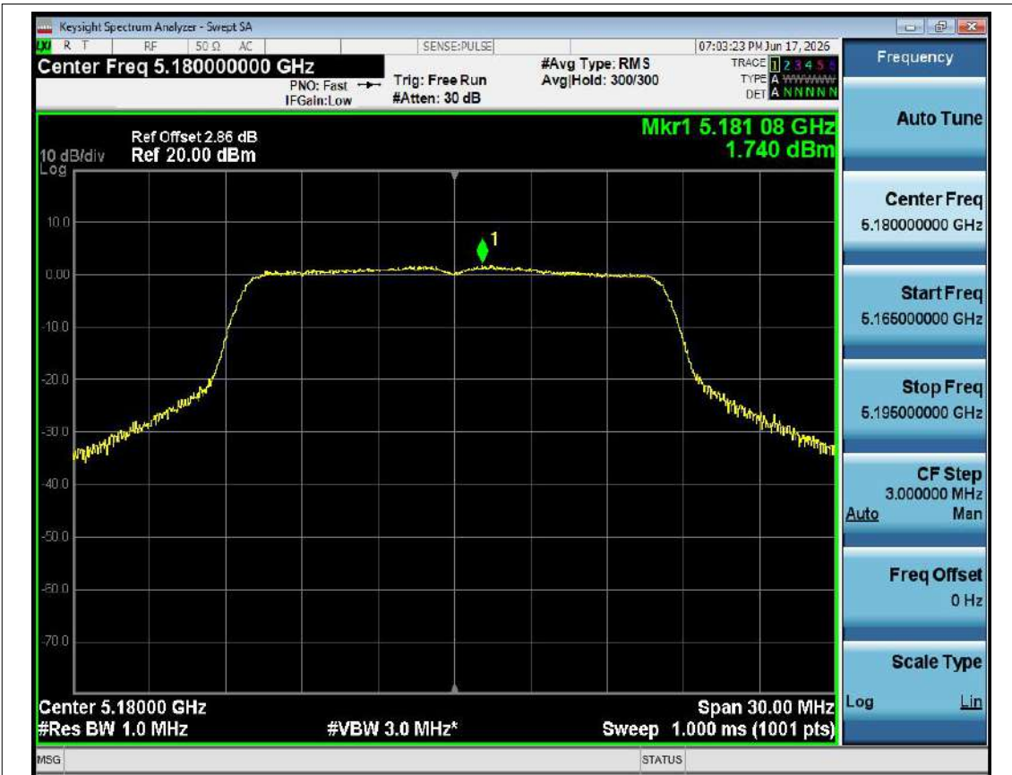
PSD NVNT a 5180MHz Ant1
