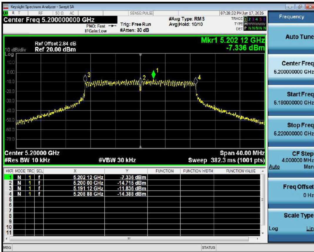
Freq. Stability NVNT n20 5200MHz Ant1
