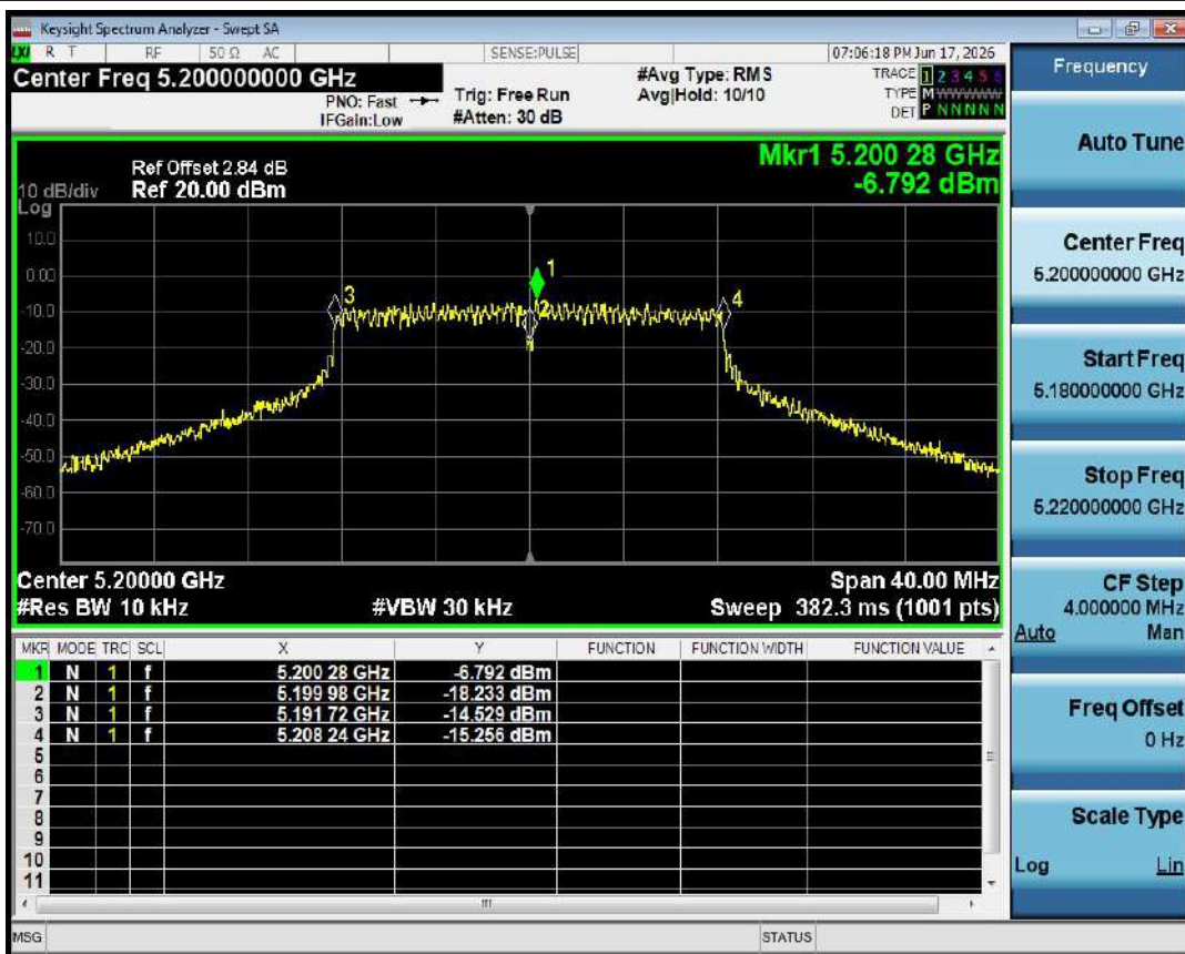
Freq. Stability NVNT a 5200MHz Ant1
