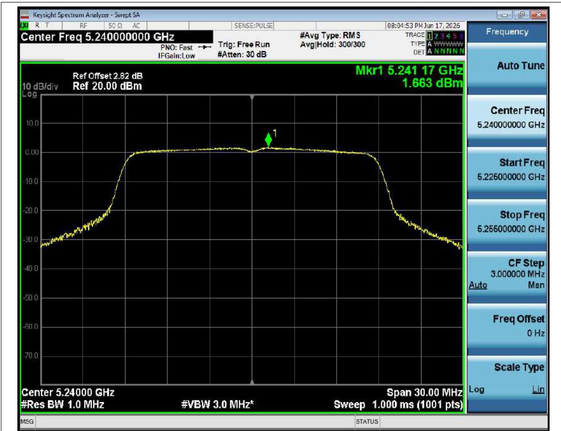
PSD NVNT ac20 5240MHz Ant1
