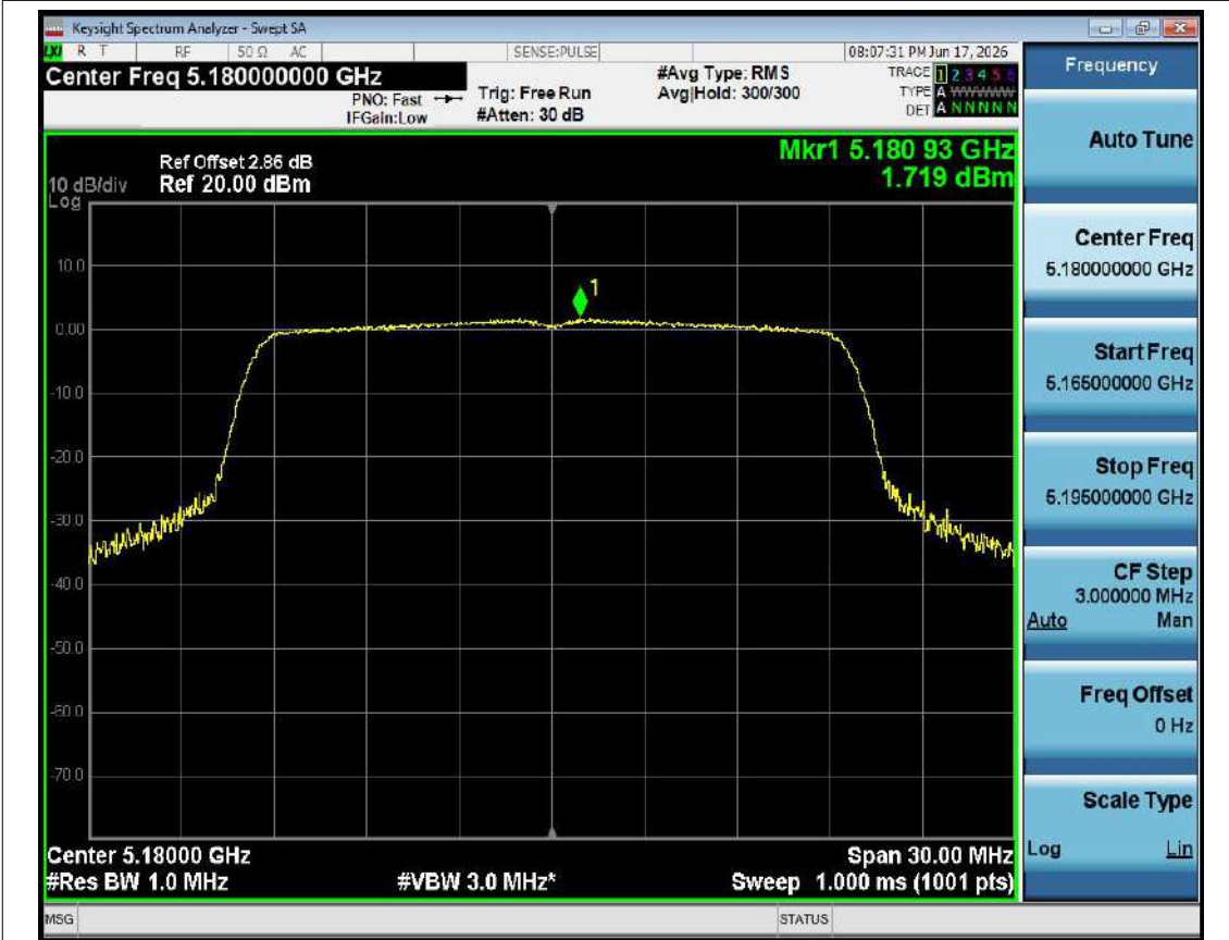
PSD NVNT ax20 5180MHz Ant1
