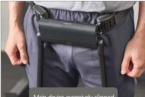
Main device excessively slipped
