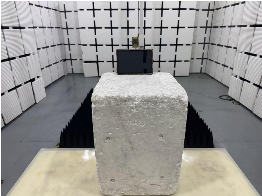
Set-up for Radiated Spurious Emission, Above 1GHz
