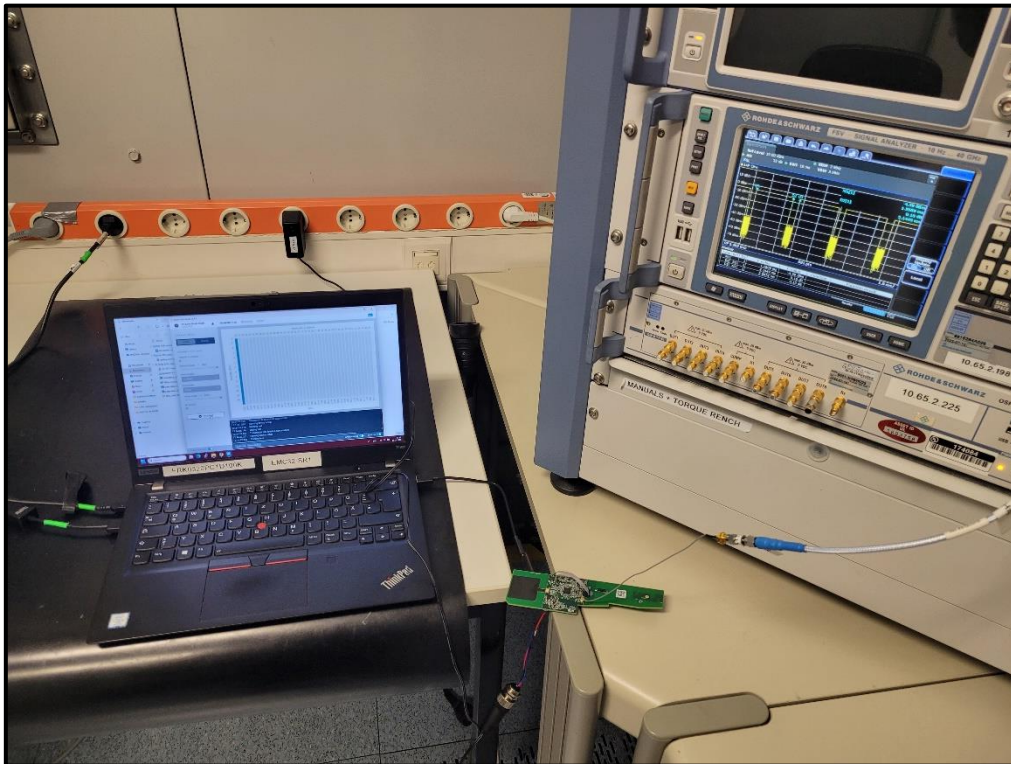
Photo 9 Conducted Test Setup
