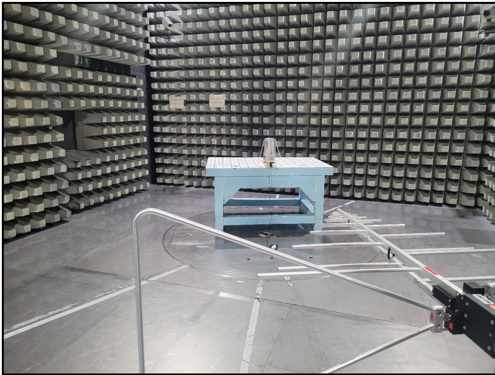
Photo 3 Radiated Test Setup from 30 MHz to 1 GHz
