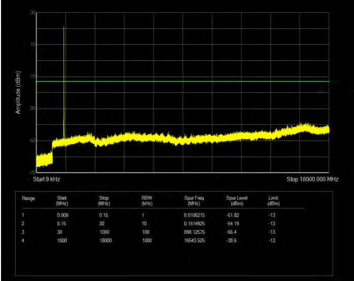
Band4 QPSK BW=5MHz Channel=20175 RB Size=1 Position=#0
