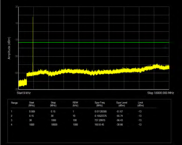
Band4 16QAM BW=1.4MHz Channel=20393 RB Size=1 Position=#0
