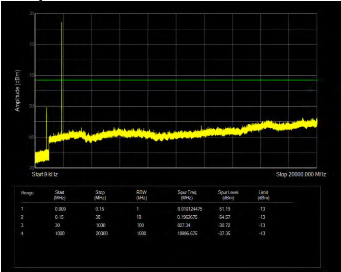
Band2 QPSK BW=3MHz Channel=19185 RB Size=1 Position=#0
