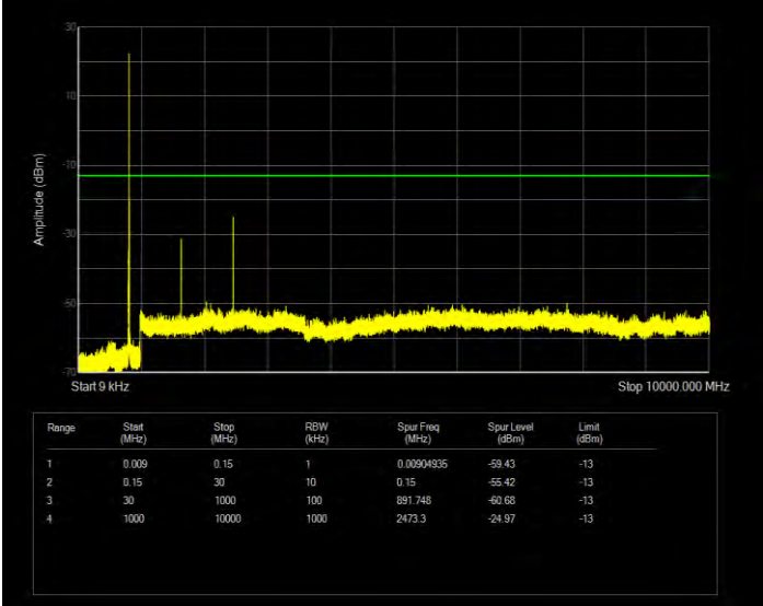
Band5 QPSK BW=3MHz Channel=20525 RB Size=1 Position=#0
