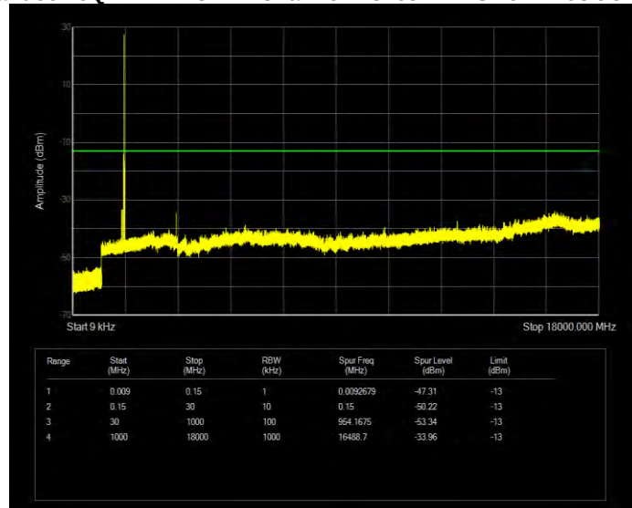
Band66 16QAM BW=5MHz Channel=131997 RB Size=1 Position=#0
