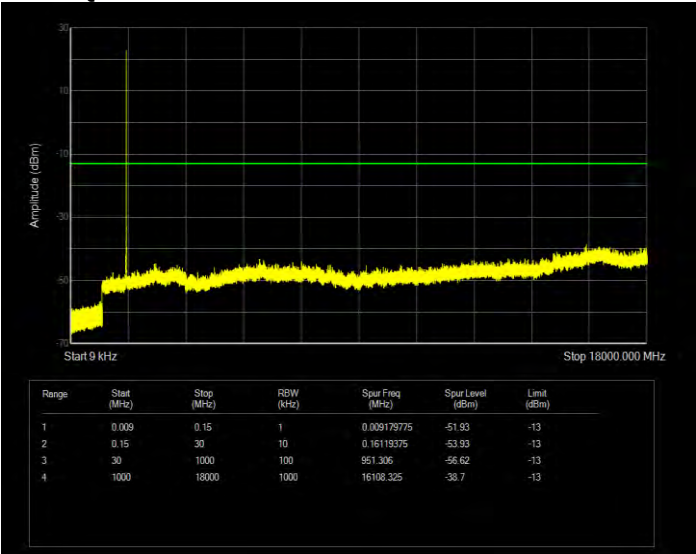
Band4 16QAM BW=1.4MHz Channel=20393 RB Size=1 Position=#0
