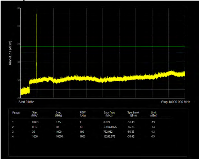
Band4 QPSK BW=5MHz Channel=20375 RB Size=1 Position=#0
