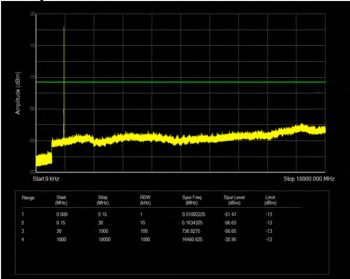
Band4 QPSK BW=3MHz Channel=20385 RB Size=1 Position=#0
