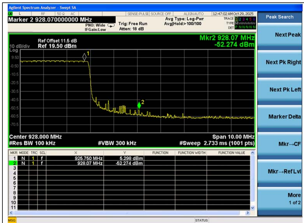
(Band edge with hopping on, Channel 64, GFSK)
