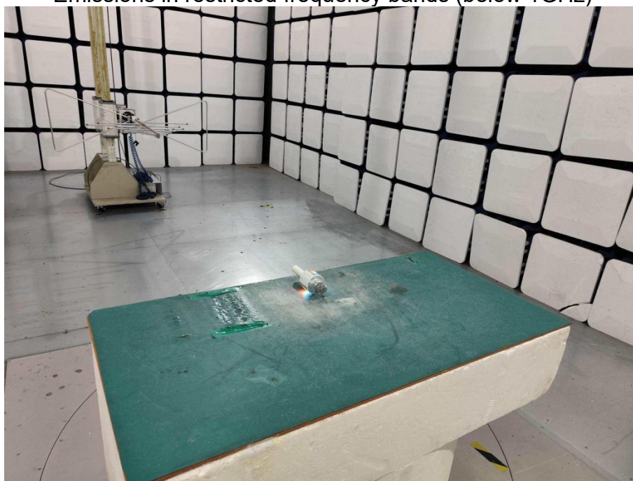
Emissions in restricted frequency bands (above 1GHz)
