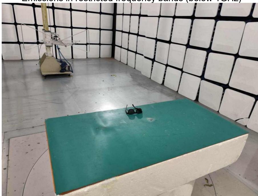
Emissions in restricted frequency bands (below 1GHz)
