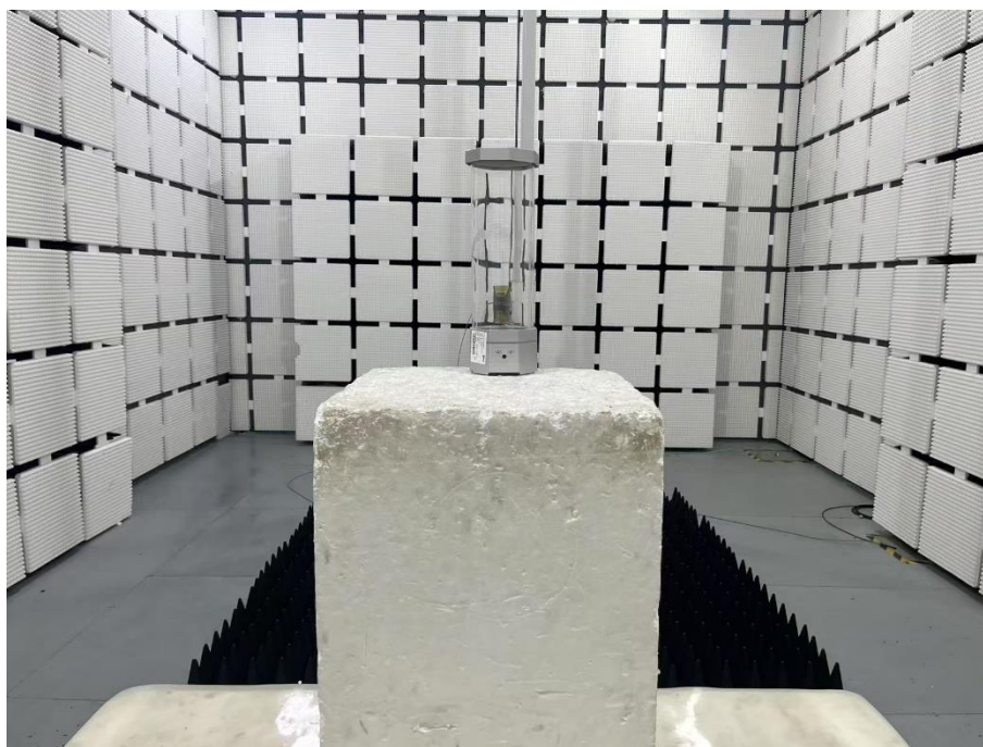
Set-up for Radiated Spurious Emission, Above 1GHz
