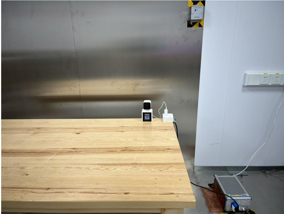
Radiated Emission Test View|(Below 1G)
