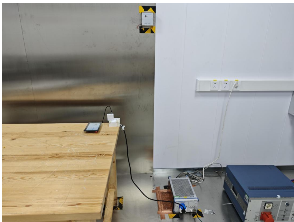
Conducted Emission Test View
