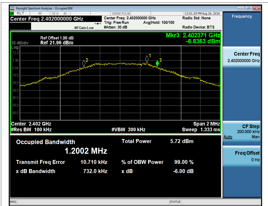
-6dB Bandwidth NVNT 2.4GHz 2402MHz Ant1
