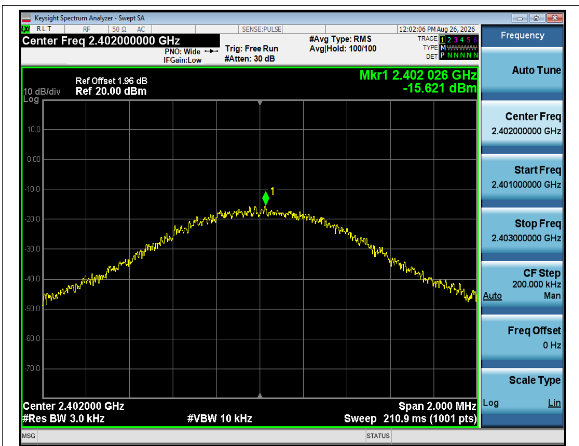
PSD NVNT 2.4GHz 2402MHz Ant1
