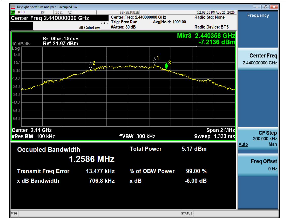
-6dB Bandwidth NVNT 2.4GHz 2440MHz Ant1
